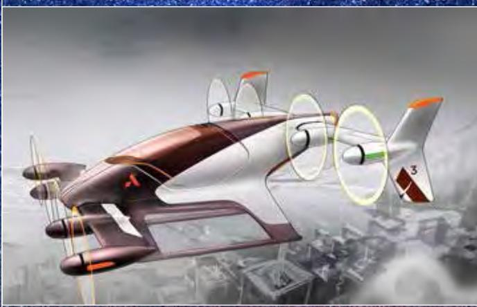
Project Vahana started in early 2016 as one of the first projects at A<sup>3</sup>, the advanced projects and partnerships outpost of Airbus in Silicon Valley. Designed to carry a single passenger or cargo, A<sup>3</sup> is aiming to make it the first certified passenger aircraft without a pilot. The aim is to fly a full-size prototype before the end of 2017, and to have a product-ready demonstrator by 2020.
