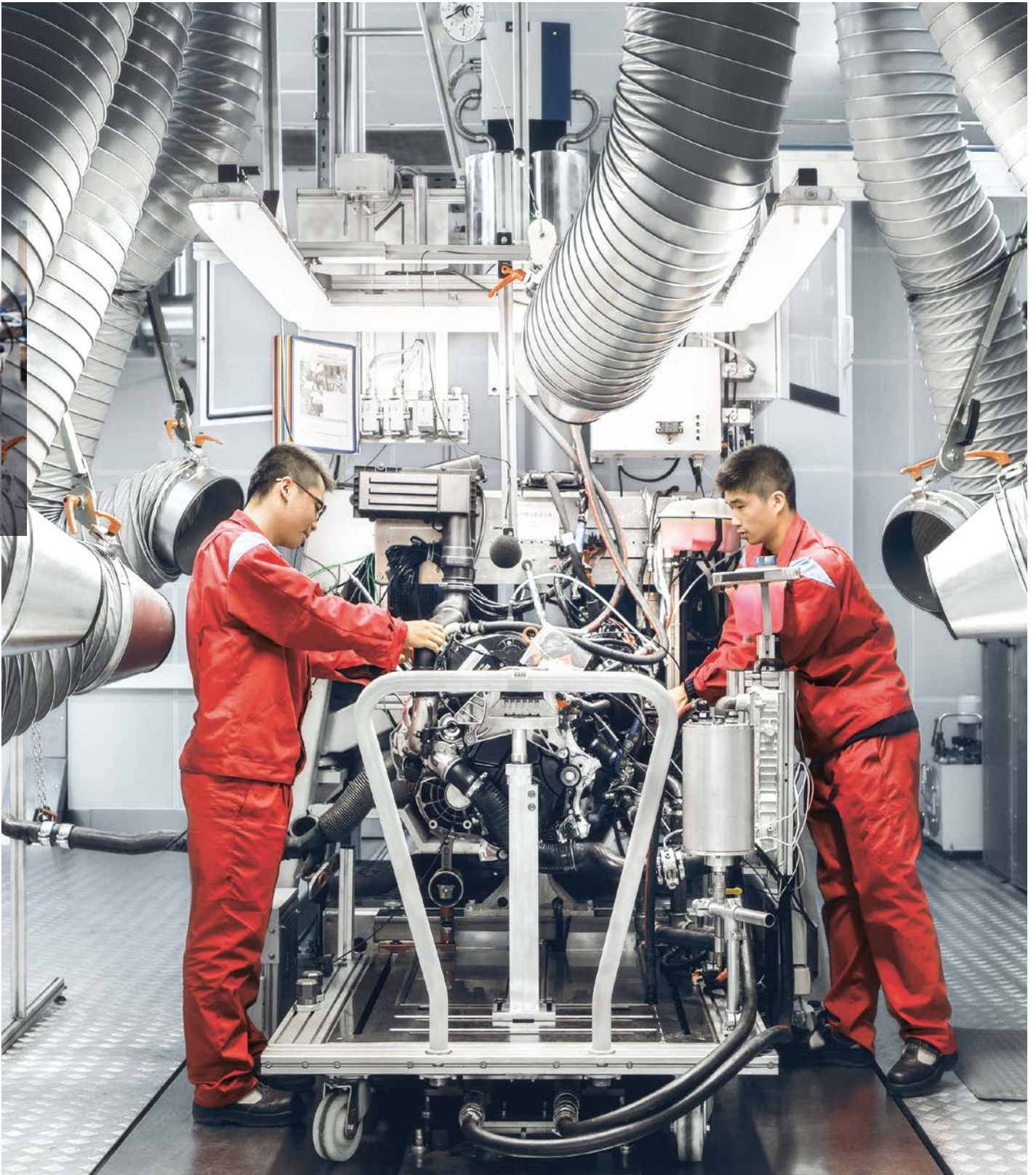
Checking and testing are part of the daily routine in the new Volkswagen FAW Engine plant – for example in the hot test room.
