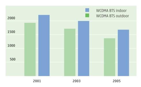
Eco-efficiency of base stations is improving. Energy consuption calculated for reference configuration inclusing three sector WCDMA base-station with each sector with 20W output power and with capacity of 64 speech channels.
