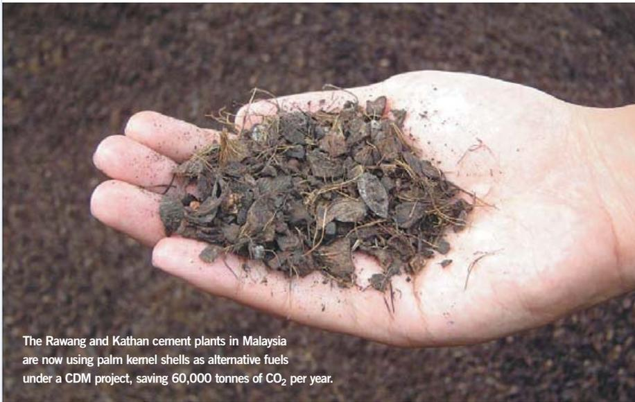
The Rawang and Kathan cement plants in Malaysia are now using palm kernel shells as alternative fuels under a CDM project, saving 60,000 tonnes of CO<sub>2</sub> per year.
