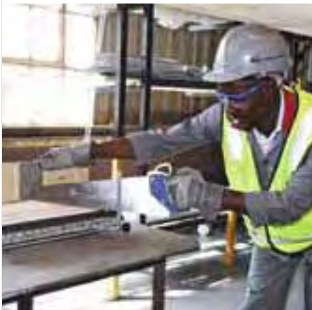
Gypsum - South Africa, Roodekop Factory and Training Center, gypsum plasterboard being sawed.
