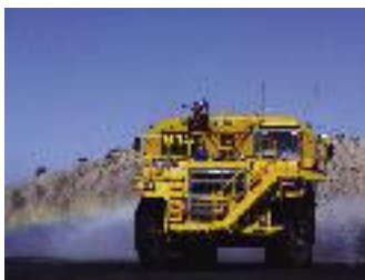
A water truck sprays water on a haul road to keep the dust levels down at Rio Tinto Coal Australia's Blair Athol mine.
