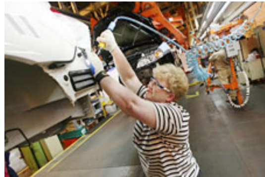
Marisel Broadwater uses a screwgun to place screws in the rear fascia quarterbracket of a Pontiac G6 at the Orion Assembly Plant in Lake Orion, Michigan.
