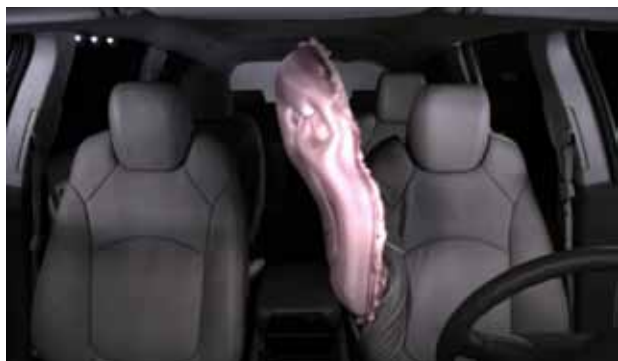
The industry's first front center air bag will help protect drivers and front passengers in far-side impact crashes where the affected occupant is on the opposite, non-struck side of the vehicle.
