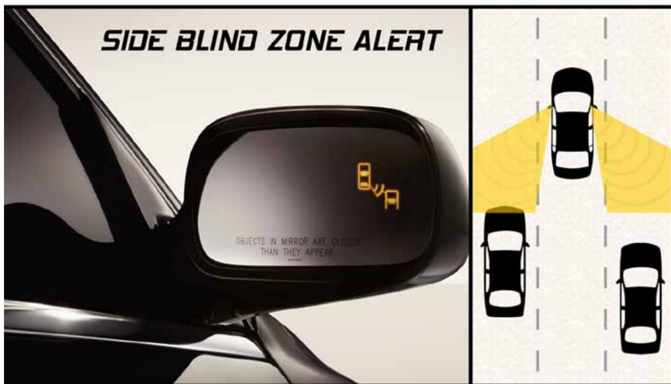
Side blind zone alert uses radar sensors to warn drivers of an object in their blind spot.
