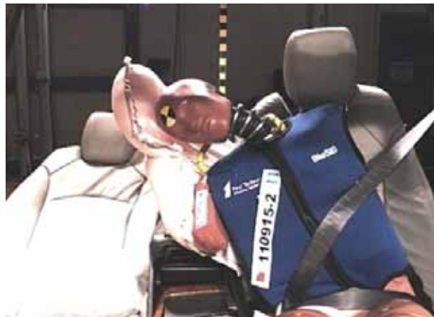
The front center air bag deploys from the right side of the driver's seat and is designed to provide restraint during passenger-side crashes when the driver is the only front occupant.
