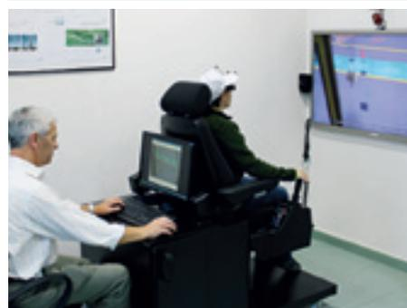
*Our Research & Development teams have developed a special simulator that uses the latest virtual reality techniques to help train crane operators. Replicating the actual experience of working the crane through state-of-the-art graphics, sound systems, LCD projectors, and movement sensors help to improve the skills of inexperienced workers, and increases safety throughout our operations.*
