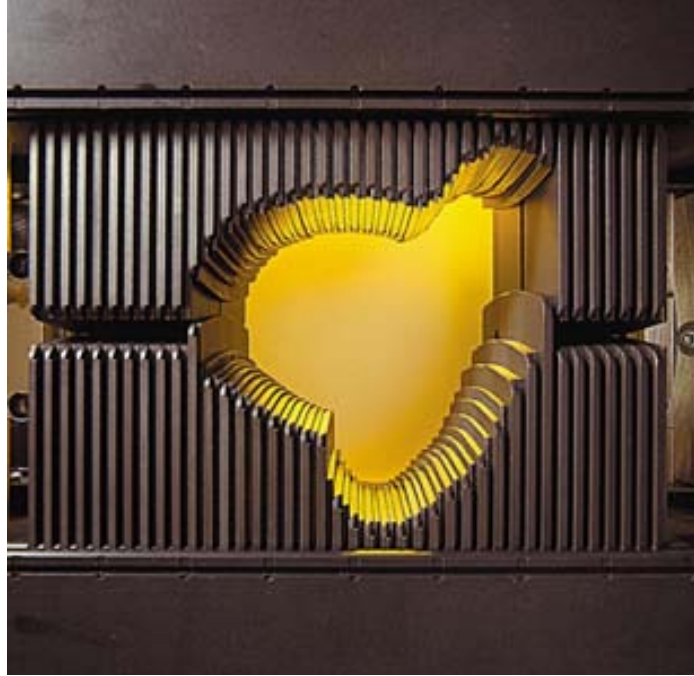
Figure 7.2. A 120 Millenium multi-leaf collimator from Varian (from the Varian webpage http://www.varian.com ).
