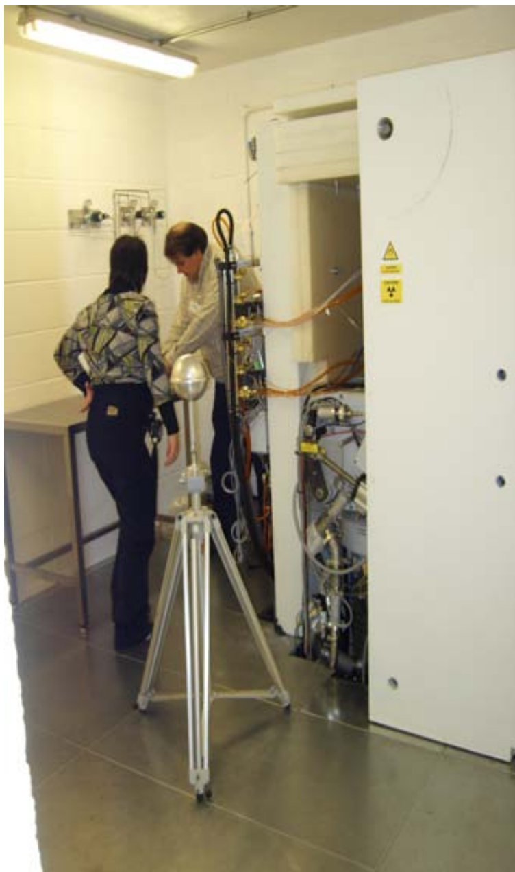
Figure 7.24. View of the GE medical system PETtrace cyclotron and of the irradiation place Point 1, situated in direct view of the target with no polyethylene shielding.
