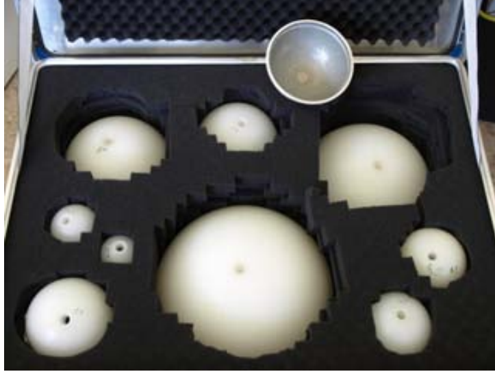
Figure 4.1. Set of polyethylene spheres and Cd shell to be used as neutron moderators with the UAB active Bonner sphere system
