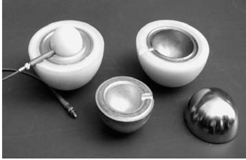
Figure 3.3. Parts of the set of modified spheres extending the PTB 'C' BSS to measurements in high energy neutron fields, taken from [36]
