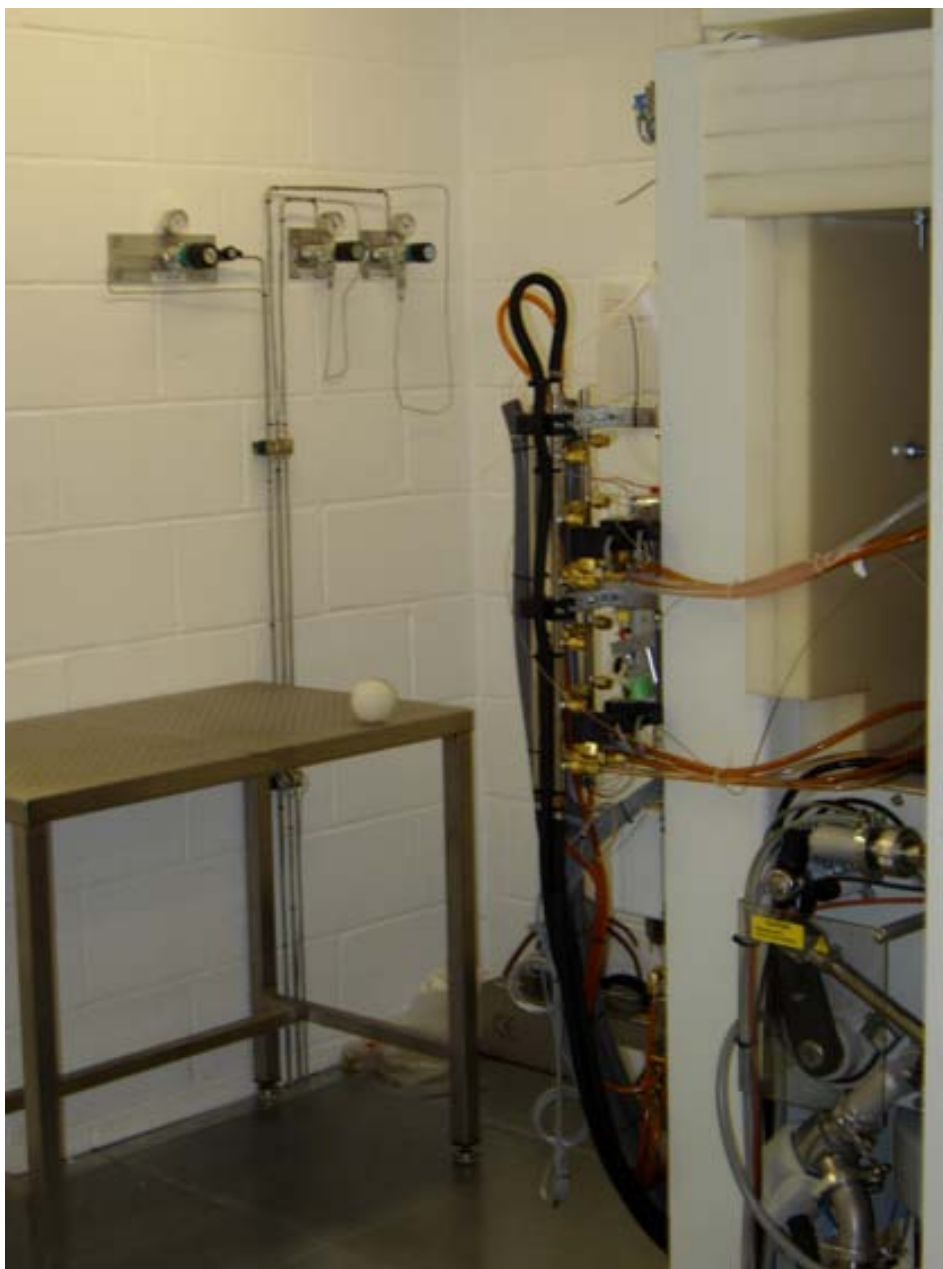
Figure 7.25. View of the GE medical system PETtrace cyclotron and of the irradiation place Point 2, situated behind the polyethylene shielding and next to target.
