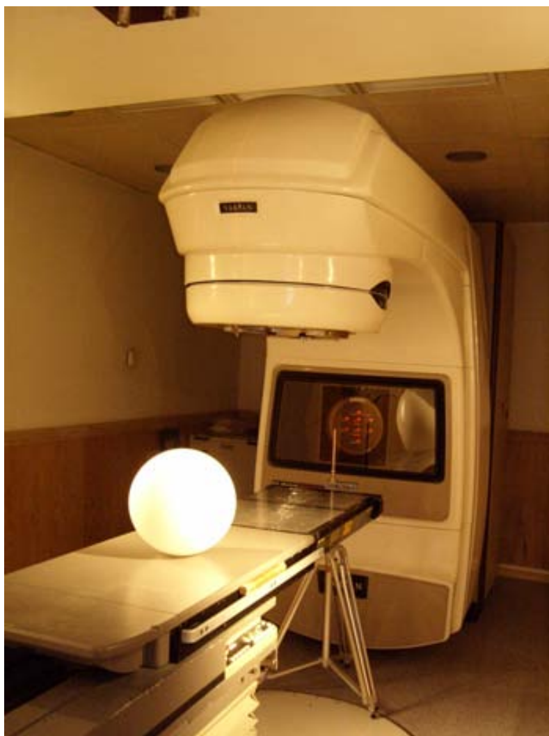
Figure 7.4. The 10 in sphere of the UAB passive BSS on the LINAC couch, prepared for exposure at 135 cm from the isocenter.
