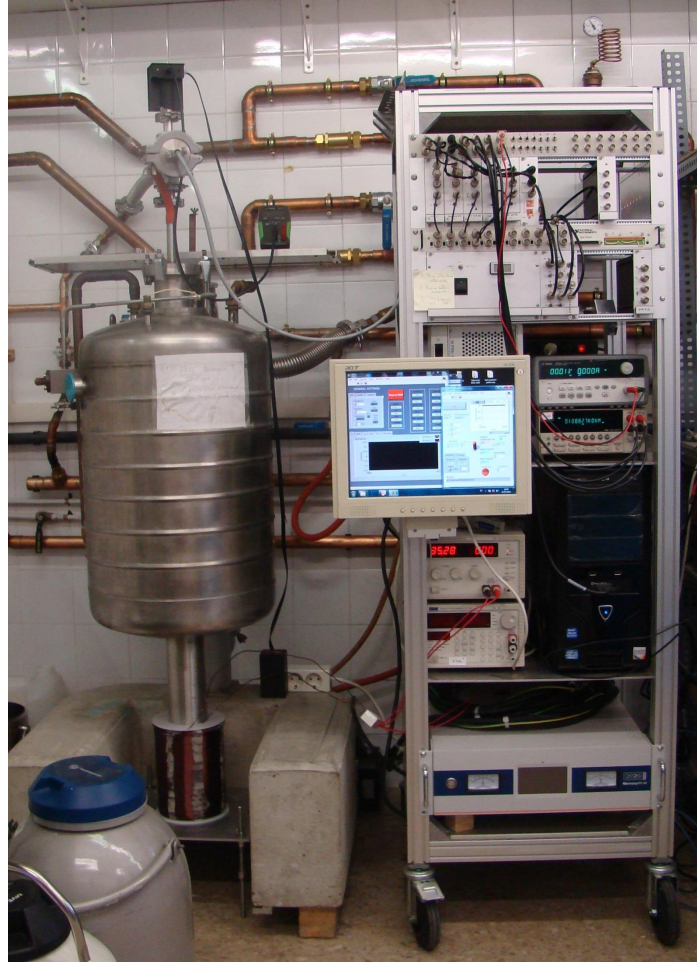
FIG. 2.11 Immersion cryostat experimental setup with the electronics dedicated to nanocalorimetry, temperature control and magnetic fields generation.
