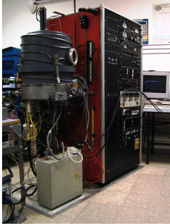
FIG. 2.7 The in-situ experimental setup consisting on a Leybold UNIVEX 450 equipped with the necessary elements to perform nanocalorimetric measurements.
