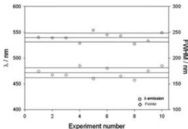
**Fig. 6** Characterization of the CdS/ZnS synthesis repeatability by the emission fluorescence wavelength and the FWHM.
