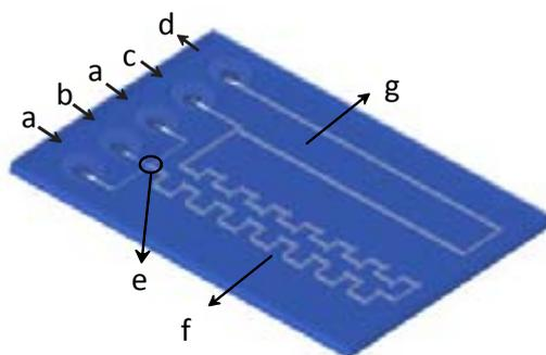
**Figure 5.3:** Schematic representation of the microfluidic platform for the synthesis of core-shell CdS/ZnS nanocrystals (**MR5**), where a: Na<sub>2</sub>S, b: Cd(NO<sub>3</sub>)<sub>2</sub>, c: Zn(NO<sub>3</sub>)<sub>2</sub>, d: outlet, e: confluence point (hydrodynamic focusing), f: three-dimensional micromixer for CdS NPs formation, g: simple microchannel for CdS/ZnS NPs synthesis.
