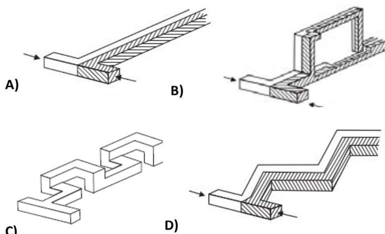
**Figure 1.2:** Most common passive micromixers. A) Basic T-shape mixer (parallel lamination). B) Join–split–join mixer (serial lamination). C) L-shape passive micromixer for mixing with chaotic advection. D) Zig-zag-shaped planar channel (chaotic advection).<sup>15-16</sup>
