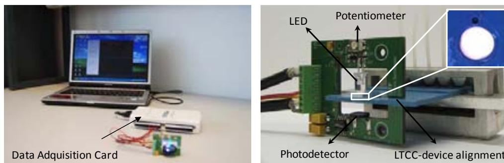
**Figure 4.21:** Images of the miniaturized optical system for monitoring the synthesis of gold nanoparticles. An image of the optical window is shown in the inner box of the right image.
