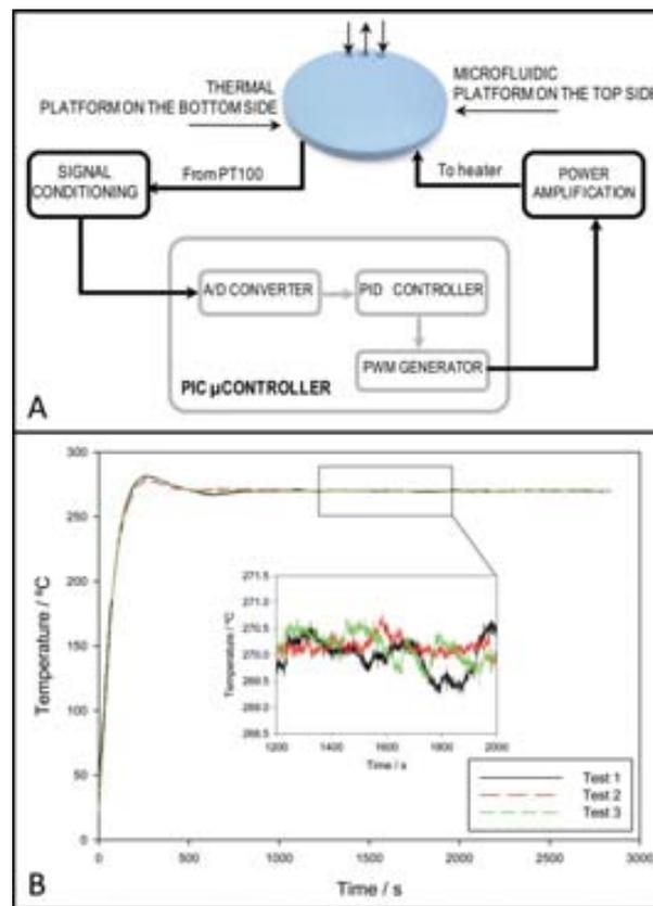
**Fig. 2** Electronics for thermal control. A: block diagram of the electronics developed for a precise digital PID temperature control. B: system responses obtained during three experiments performed at a set-point of 270 °C once the PID parameters were optimized. Small variations in the order of  $\pm 0.5 \text{ } ^\circ\text{C}$  were observed.
