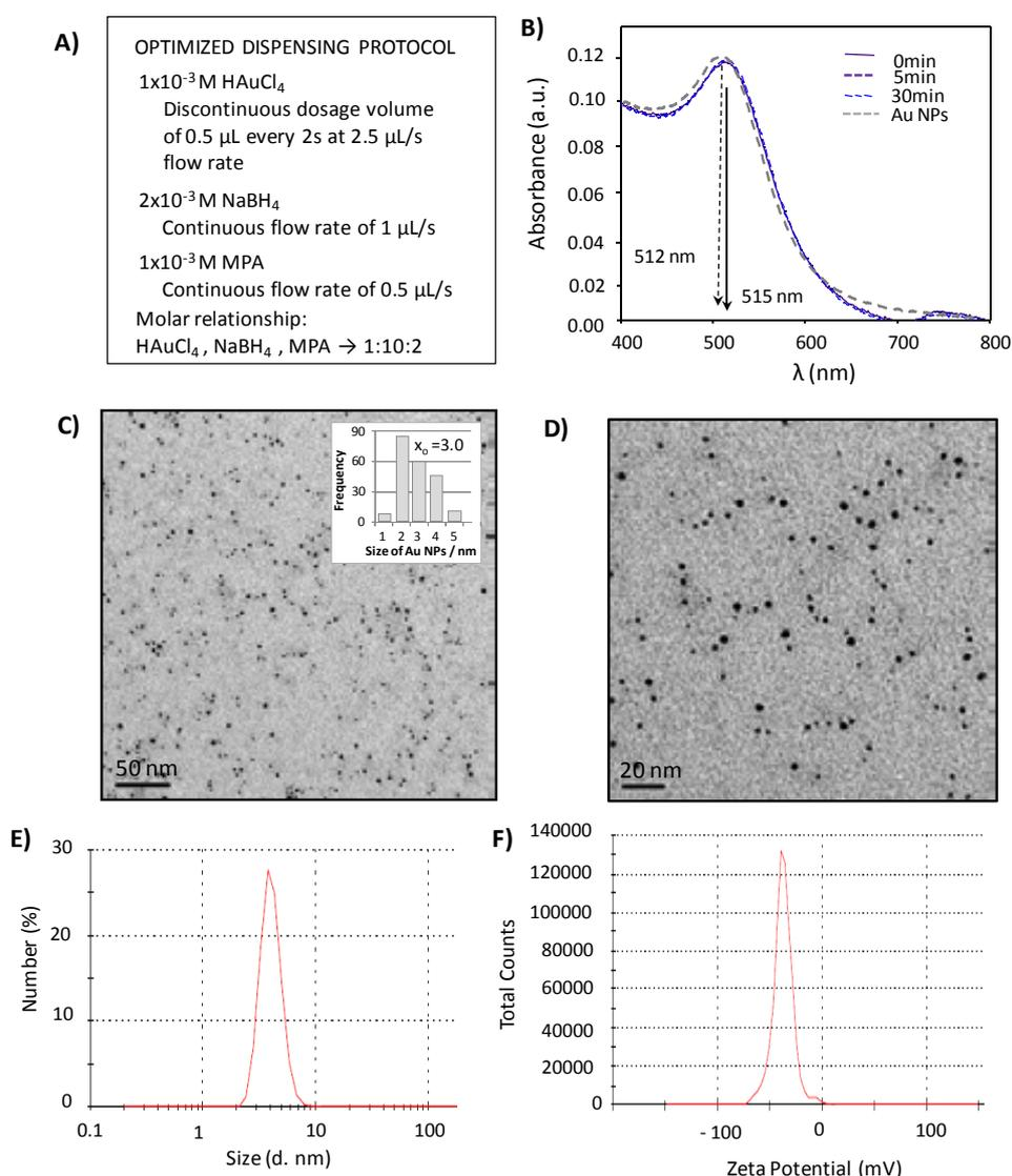
**Figure 4.17:** Results from the MPA stabilized Au NPs, obtained in the MR3 microreactor. **A)** Optimized chemical and hydrodynamic parameters. **B)** UV-Vis spectra recorded with time and its comparison with Au NPs. **C)** and **D)** TEM images and its correspondent histogram. **E)** DLS spectrum. **F)**  $\zeta$  potential measure.
