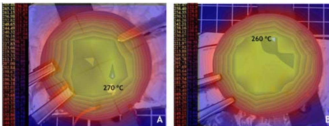
**Fig. 6.** Isothermal maps obtained on the bottom (A) and the top (B) of the monolithic microsystem. Punctual temperature measurements in the zone of the sensor are indicated (set point of the control system: 270 °C).
