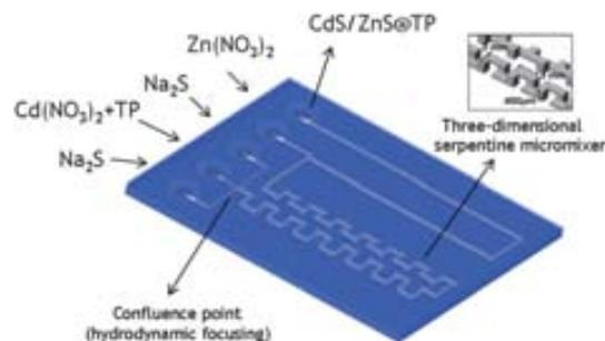
**Fig. 3** The ceramic microreactor design for the synthesis of core-shell nanocrystals, incorporating the concept of hydrodynamic focusing, a three-dimensional serpentine micromixer for the formation of the core quantum dots and a longitudinal channel for the shell formation.
