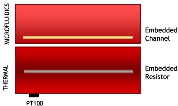
**Fig. S.2** Schematic diagram of the temperature analysis developed to estimate temperature in the microfluidic channel.
