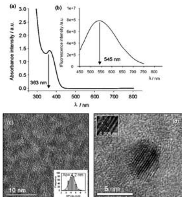
**Fig. 5** (a) UV-vis and (b) fluorescence emission spectra of the obtained CdS/ZnS nanocrystals, (c) a TEM image of the obtained quantum dots using the ceramic microreactor and (d) a HRTEM image with the lattice fringes highlighted.
