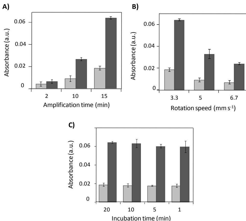
**Figure 6.15:** Signals obtained from the different experiments performed during the optimization of the microsystem ( $n=3$ ). **(A)** Amplification time, **(B)** rotation speed and **(C)** incubation time of the assay. Dark bars show the absorbance signal for a 20 nM *E. coli* target. Light bars are blank signals.
