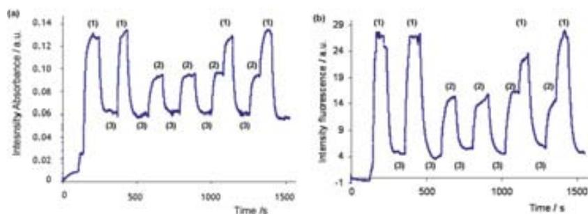
**Fig. 7** Absorbance (a) and fluorescence emission (b) graphics recorded using the miniaturized optical system at different flow rates; 0.5  $\mu\text{L}$  (cadmium dosage volume 1), 0. 25  $\mu\text{L}$  (dosage volume 2) and 0.08  $\mu\text{L}$  (dosage volume 3).
