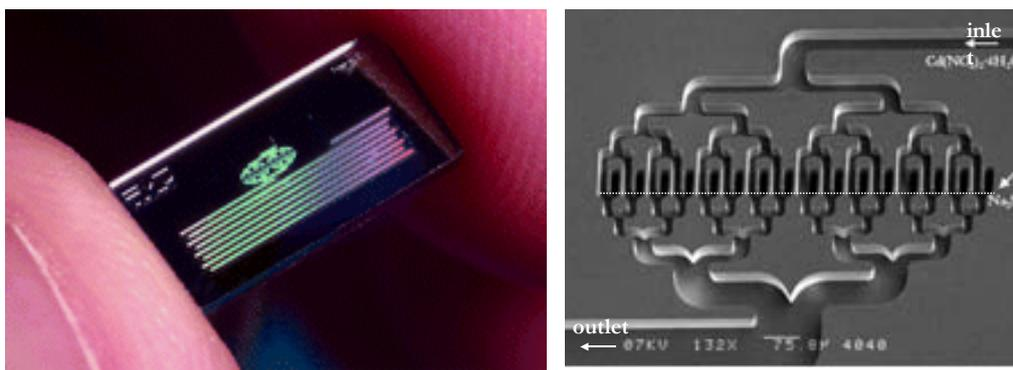
**Figure 1.48:** Image from the first microreactor for the synthesis of CdS nanoparticles. After mixing the channels, where sodium sulfide and cadmium nitrate are supplied, particles are formed in another microfluidic channel.<sup>396</sup>
