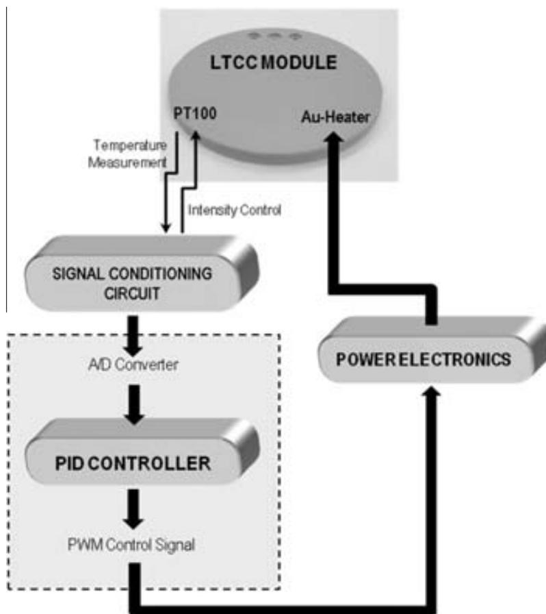
Fig. 3. Block diagram of the digital/analog electronics for an accurate control of temperature inside the microreactor.
