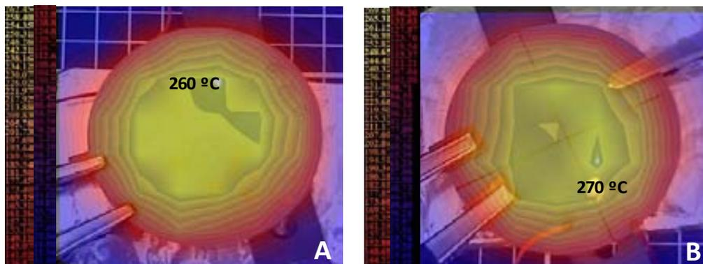
Nevertheless, from the obtained results it can be concluded that, using either of both configurations, reagents are exposed to specific, uniform and controlled temperature levels provided by the thermal platform during their flow through.
