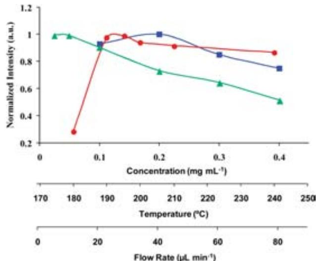
**Fig. 2** Optimization of the chemical and hydrodynamic parameters for the synthesis of Cdots in the ceramic microfluidic system ( $\lambda_{\text{exc}} = 325$  nm,  $\lambda_{\text{em}} = 420$  nm). Red circles: temperature (°C), blue squares: concentration (μg mL<sup>-1</sup>), green triangles: flow rate (μL min<sup>-1</sup>).
