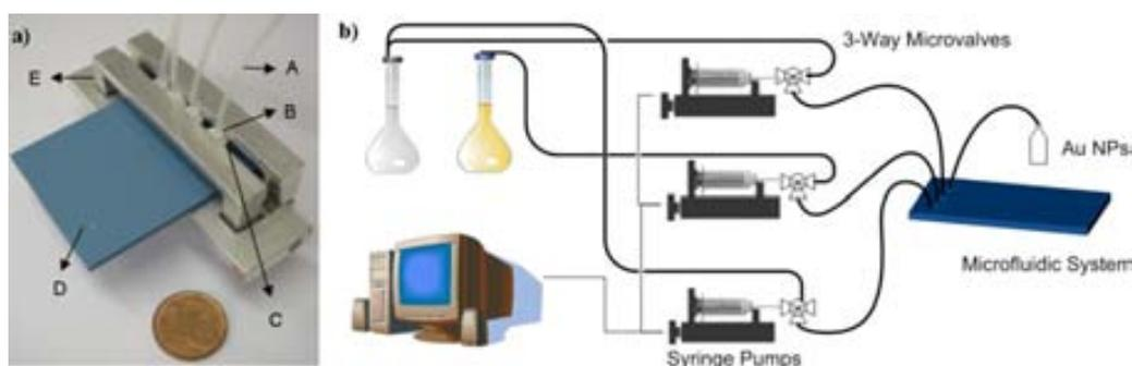
**Figure 1.** (a) Simple user-friendly connection system, designed to attach the microfluidic device with the PTFE tubes. A: PTFE tubes, B: PTFE cones, C: o-rings, D: LTCC microreactor, E: connection piece. (b) Diagram of the entire flow microsystem setup for the synthesis of Au NPs.
