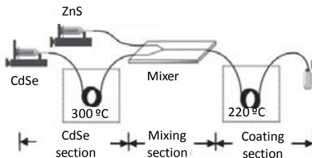
**Figure 1.50:** Scheme of sequential microreactor for the synthesis of core-shell CdSe/ZnS quantum dots.<sup>409</sup>
