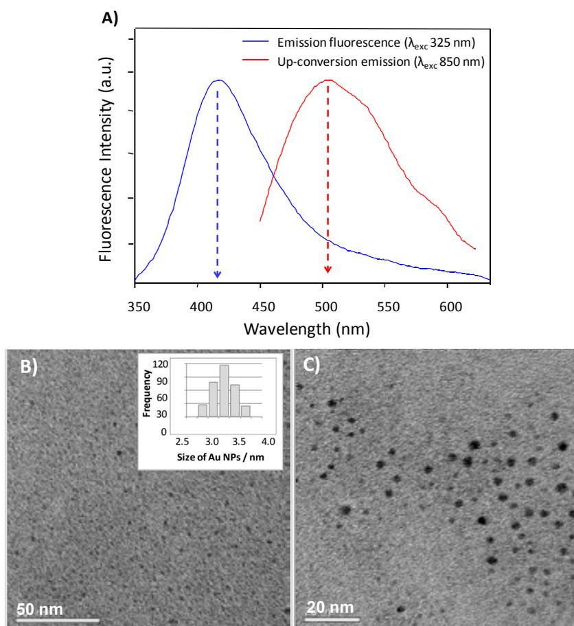
**Figure 5.31:** Characterization of the Cdots synthesized in **MR7**. **A)** Fluorescence emission spectra by UV (blue) and NIR (red) excitation. **B** and **C)** TEM images with the size-histogram and the calculated average size. **D)** HRTEM image and an amplification with the lattice fringes highlighted. **E)** SAED pattern of the nanoparticles.
