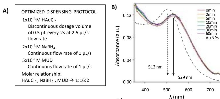
**Figure 4.18:** Results from the MUD stabilized Au NPs, obtained in the MR3 microreactor. **A)** Optimized chemical and hydrodynamic parameters. **B)** UV-Vis spectra recorded with time and its comparison with Au NPs.
