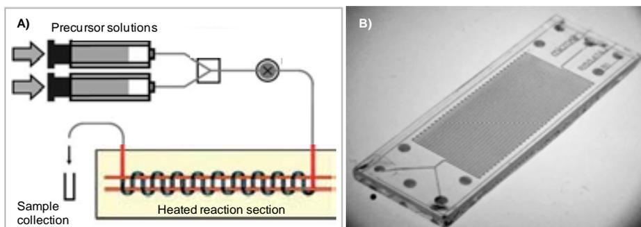
Examples of sequential synthesis involve the use of segmented or single flow, such as the scheme shown in figure 1.50, where sequential reactions in separate microreactors take place.<sup>409</sup>
