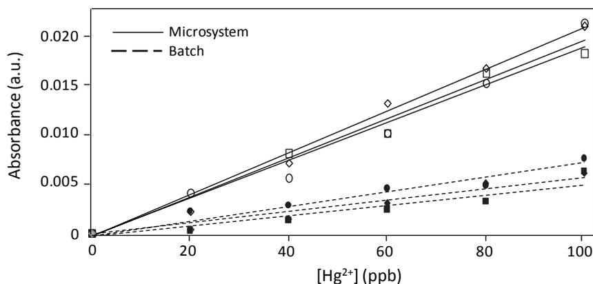
**Figure 6.11:** Calibration curves obtained with the polymeric microfluidic platform and its comparison with the previously obtained in batch.
