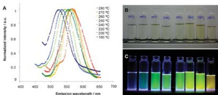
**Fig. 3** A: fluorescence emission spectra of the nanocrystals synthesized in the microreactor from 180 to 280 °C with a molar ratio of Cd : Se 1 : 10. B: images of the obtained QDs colloidal solutions, highly diluted with chloroform, from the different tested range of temperatures under room and UV (C) light.
