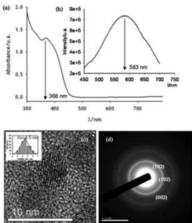
**Fig. 2** (a) UV-vis and (b) fluorescence emission spectra, (c) a HRTEM image and (d) a SAED pattern of CdS nanocrystals synthesized in the microreactor.
