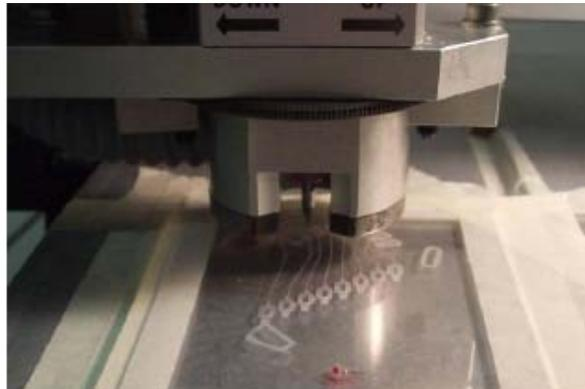
The CNC integrates a high precision micrometer, which enables defining the depth in the course of the micromachining. In order to protect the steel base of the equipment, a sacrificial timber is placed over the working area, fixing the substrate material by means of two metal pins located along the axis of the base. Polymeric layers are located over the sacrificial timber.
