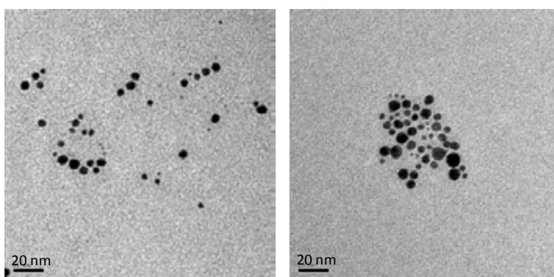
**Figure 4.6:** TEM images from silver NPs synthesized with **MR1F** ceramic microfluidic system. The hydrodynamic and chemical parameters consisted on 5 mM  $\text{NaBH}_4$  solution continuously pumped at  $1 \mu\text{L s}^{-1}$  syringe flow rate, and 1 mM  $\text{AgNO}_3$  at  $1 \mu\text{L s}^{-1}$ .
