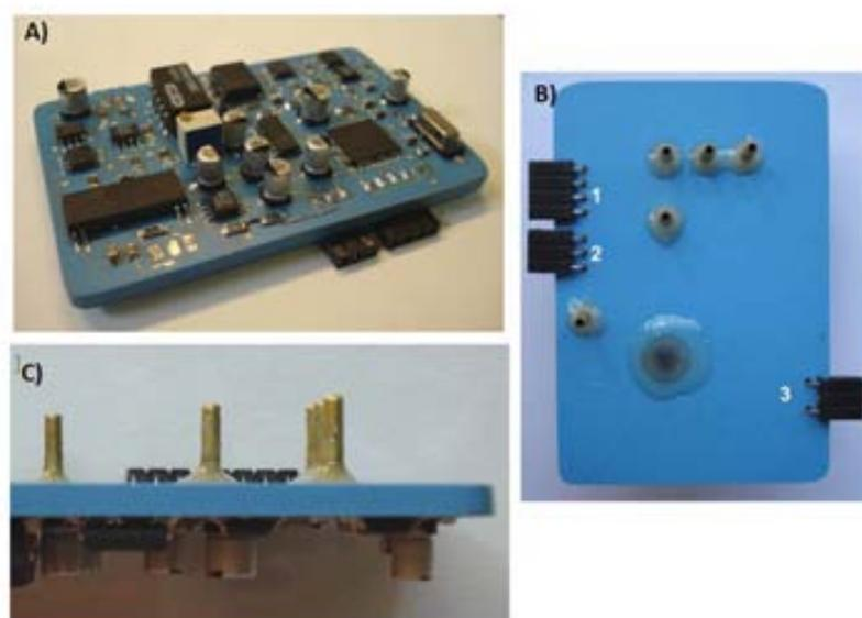
**Figure 1.6:** Ceramic microfluidic chip for potentiometric measurements, which integrates the fluidics and electronics in a single device. **A)** Bottom view of the monolithic with the electronics for data acquisition and digital signal processing. **B)** Top view of the microanalyzer. Fluidics and the detection system are integrated on this side. **C)** Lateral view of the device.<sup>27</sup>
