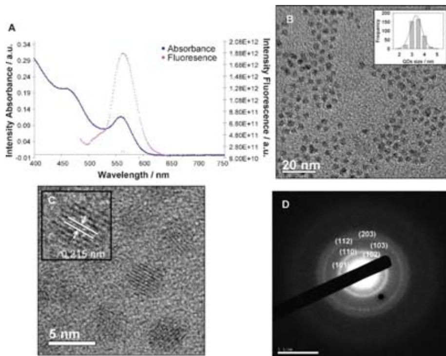
**Fig. 4** A: absorption (in blue) and fluorescence emission (in pink) spectra of the CdSe quantum dots synthesized in the microreactor at 270 °C. TEM image (B), HRTEM image (C) with the lattice fringes highlighted, and SAED pattern image (D) of the obtained CdSe quantum dots.
