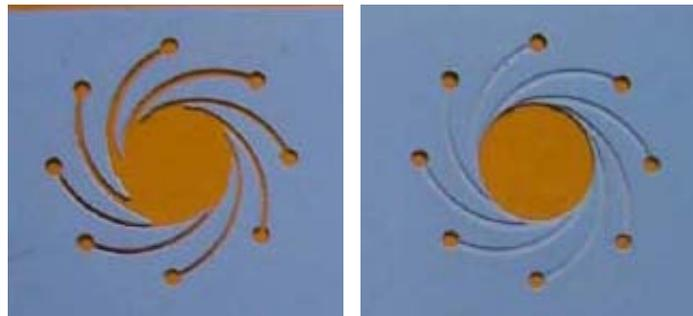
In some applications, where roughness is highly important such as in bioanalytics, where unspecific adsorption of biological materials increases with the roughness of the material, the use of a different patterning technique, such as hot-embossing is preferable approaches to minimize surface irregularities.
