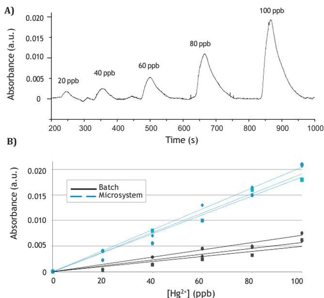
**Fig. 7.** (A) Example of the obtained signal from a mercury (II) calibration. (B) Comparison of the calibration curves obtained with the batch procedure and using the microfluidic system at the low concentration range.
