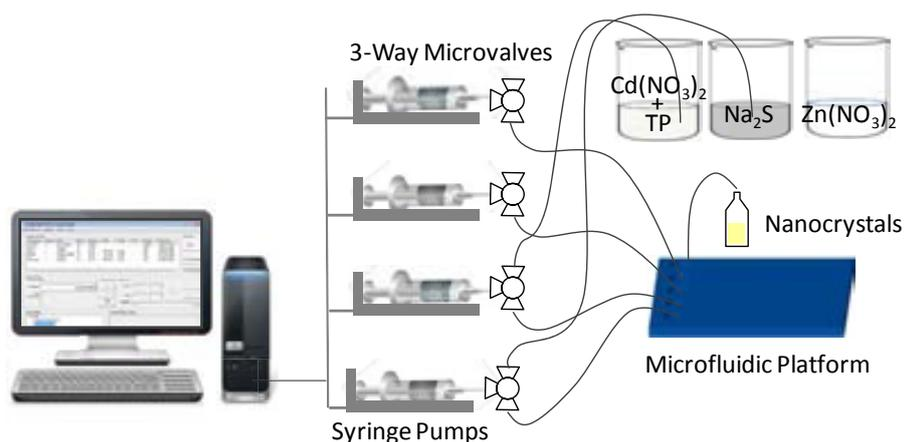
**Figure 5.1:** Microsystem set-up for the synthesis of CdS/ZnS core-shell nanoparticles.
