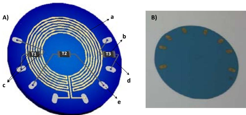
The characterization of the circular resistor by means of the thermocouple showed a radial and more uniform distribution of the temperature when a certain and constant voltage is applied. A more accurate characterization was also done, which involved the measure of the temperature in a concrete point of the heater when increasing the voltage. As it can be observed in figure 5.12, a linear response was obtained in all cases.
