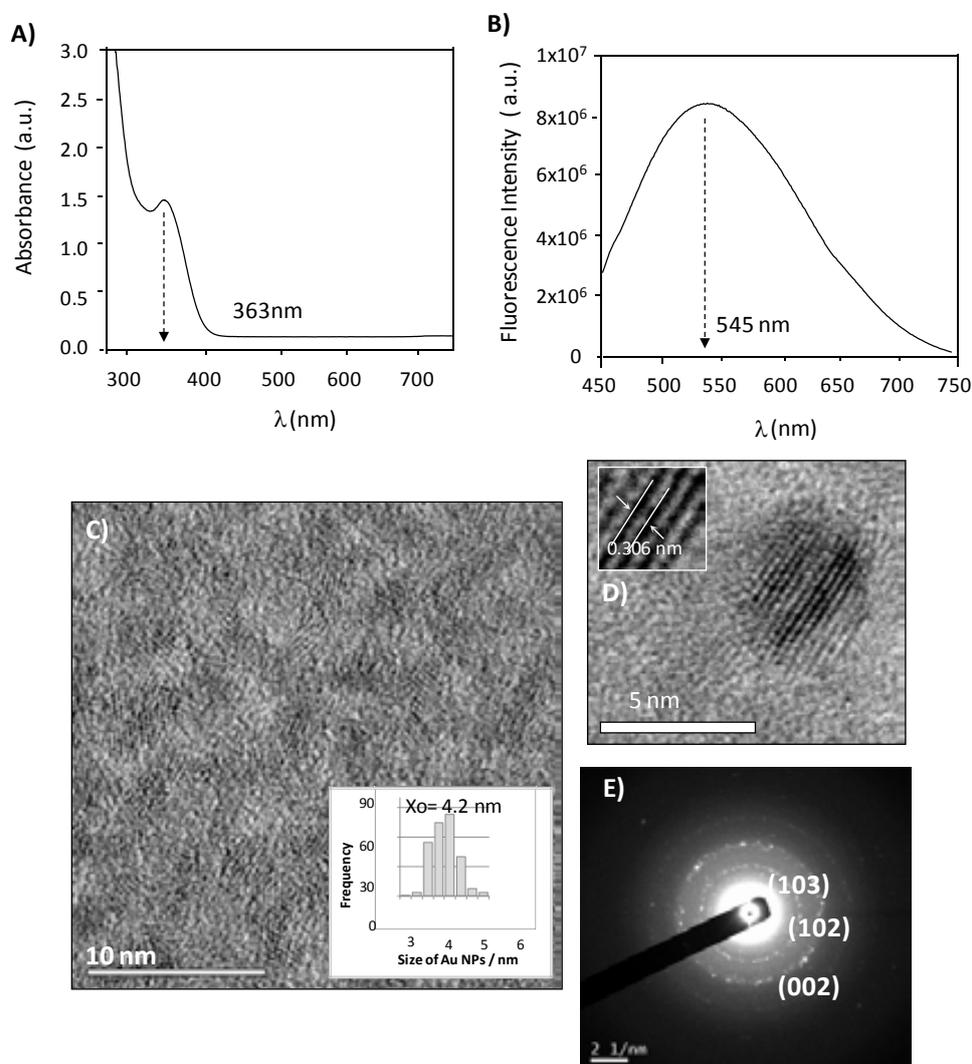
**Figure 5.5:** Characterization of the CdS/ZnS nanocrystals synthesized in MR5 at the optimized conditions. **A)** UV-Vis spectrum. **B)** Emission fluorescence spectrum. **C)** TEM image and its correspondent histogram. **D)** HRTEM image. **E)** Electron diffraction (SAED) pattern of the selected area.
