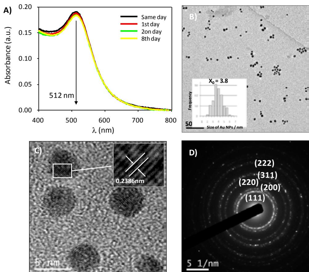
**Figure 4.13:** Characterization of the Au NPs synthesized in the MR2G ceramic microreactor at the optimized conditions. **A)** UV-Vis spectra recorded with time. **B)** TEM image and its correspondent histogram. **C)** HRTEM image with its lattice fringes. **D)** Electron diffraction (SAED) pattern of the selected area. **E)** DLS spectrum. **F)**  $\zeta$  potential measure.
