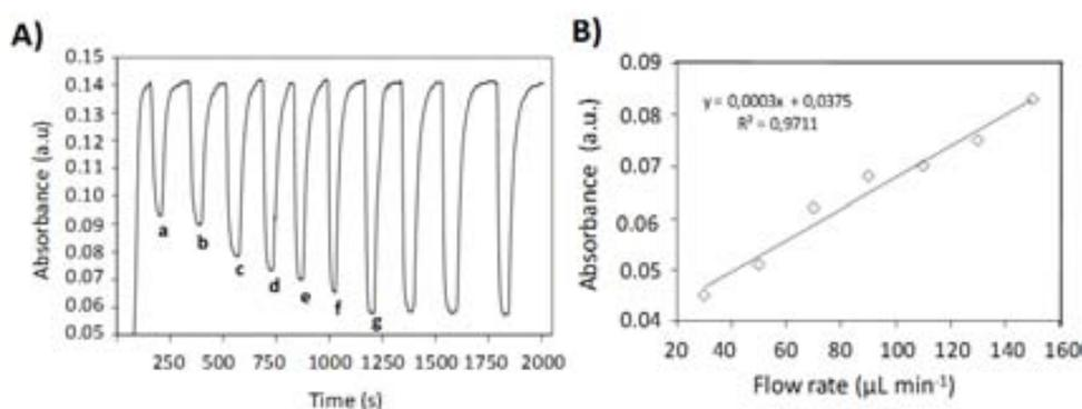
**Figure 4.22:** Signal recording (A) and obtained calibration curve (B) for the dilution of gold nanoparticles at different flow rates of water; a:  $30 \mu\text{L min}^{-1}$ , b:  $50 \mu\text{L min}^{-1}$ , c:  $70 \mu\text{L min}^{-1}$ , d:  $90 \mu\text{L min}^{-1}$ , e:  $110 \mu\text{L min}^{-1}$ , f:  $130 \mu\text{L min}^{-1}$ , g:  $150 \mu\text{L min}^{-1}$ .
