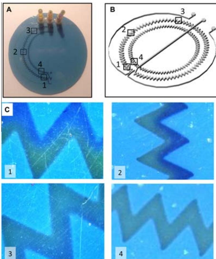
**Fig. 4.** Fluidic/hydrodynamic qualitative visual characterization of the microfluidic system. (A) Picture of the open to air microfluidic platform covered with a polymeric foil. (B) Three-dimensional inner view of the microfluidic platform. (C) Photographs corresponding to frames at different points of the micromixer.
