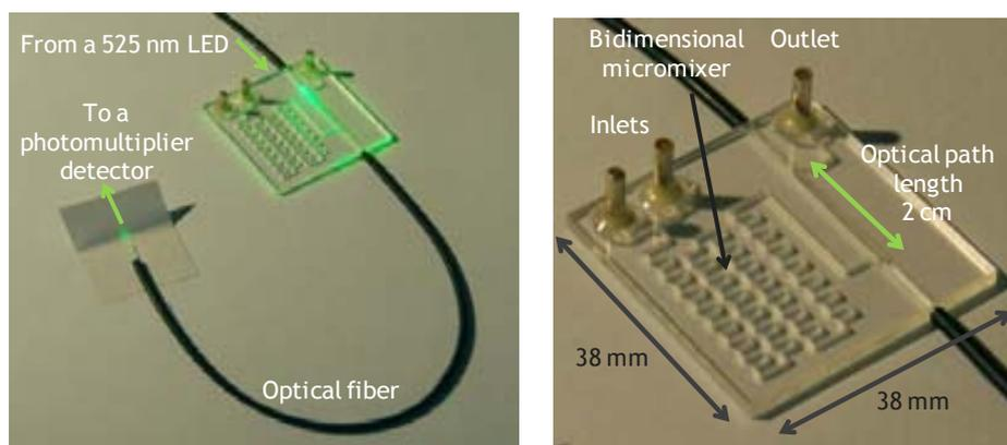
**Figure 6.8:** Images of the microfluidic platform constructed for the continuous monitoring of mercuric ion.
