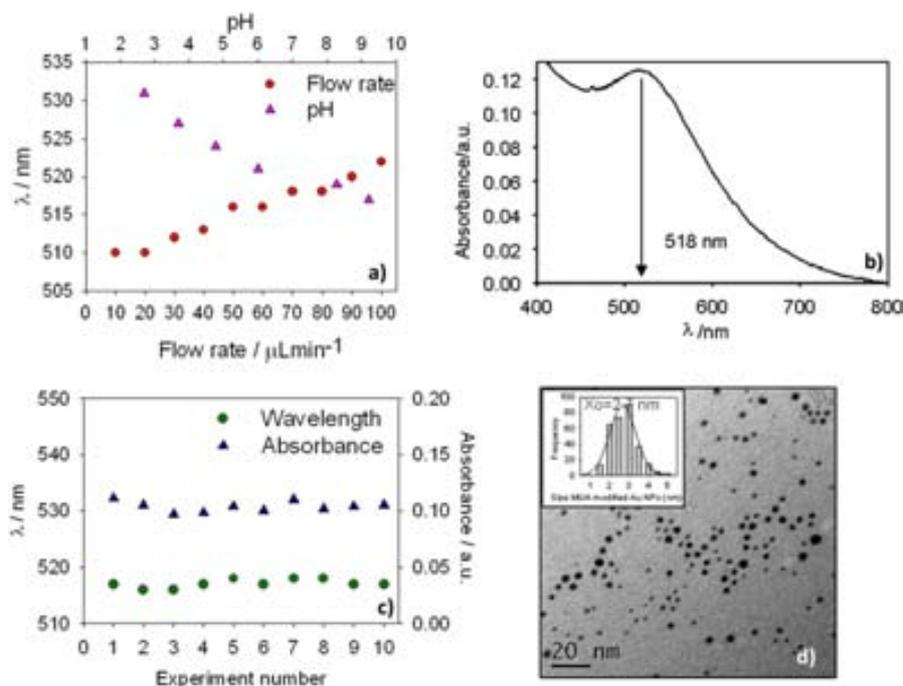
**Figure 4.** Results from the MUA Au NPs, obtained in the ceramic microreactor. (a) Study of the effect of pH and MUA flow rate on the SPR band position. (b) UV-vis spectra from the synthesized modified Au NPs using the optimized experimental conditions. (c) Characterization of the synthesis repeatability of the modified AuNPs following the position and the intensity of the SPR band. (d) TEM image from the obtained 2.7 nm NPs.
