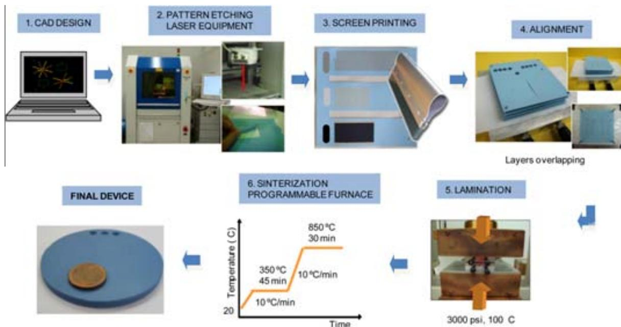
Fig. 1. Fabrication procedure of the LTCC microsystems.
