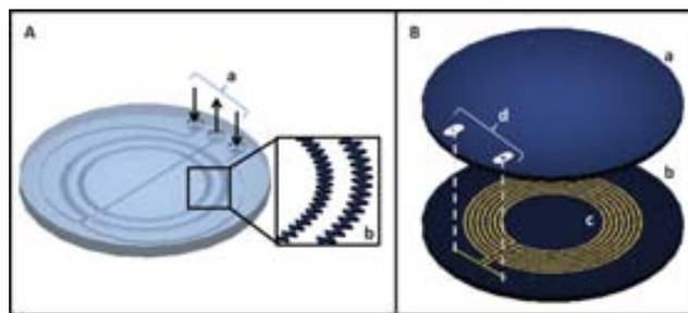
**Fig. 1** LTCC-based microsystem for CdSe quantum dots synthesis (6 mm diameter and 2 mm depth). A: microfluidic platform; a: inlets/outlet; b: amplification of a microreactor region. B: thermal platform showing the embedded heater; a: cover of the heater; b: base where heater was screen-printed; c: embedded gold-based heater; d: pads for external electronic control.
