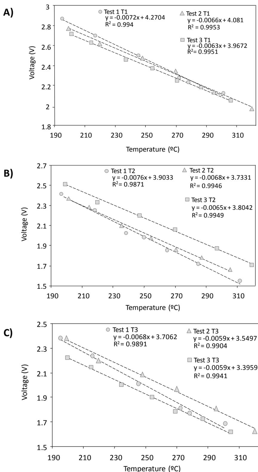
**Figure 5.13:** Characterization of thermistors. The different calibration curves (by triplicate) represent the variation of the voltage in the electronic circuit with the temperature. **A) Thermistor 1. B) Thermistor 2. C) Thermistor 3.**
