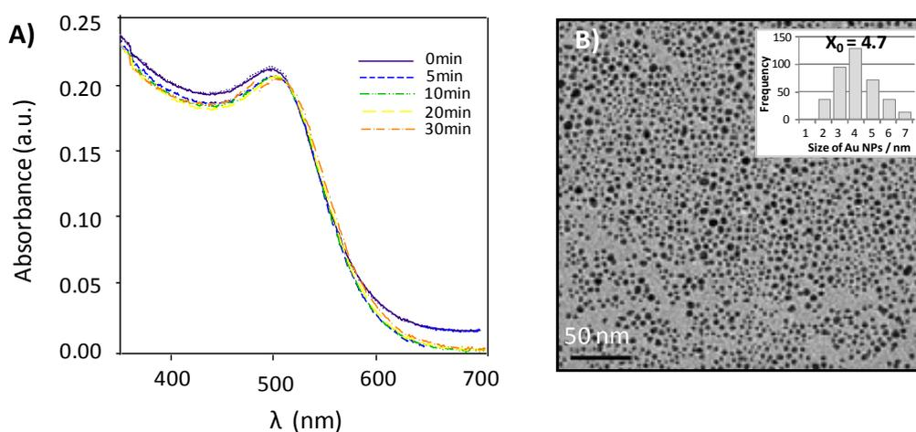
**Figure 4.11:** UV-Vis spectra and TEM images from Au NPs synthesized with **MR1D** ceramic microfluidic systems. The hydrodynamic and chemical parameters consisted on 3 mM  $\text{NaBH}_4$  solution pumped at  $2 \mu\text{L s}^{-1}$  syringe flow rate, and 2.5 mM  $\text{HAuCl}_4$  at  $1 \mu\text{L s}^{-1}$ .
