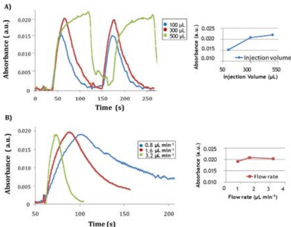
**Fig. 6.** Hydrodynamic parameters optimization of the microfluidic system for 100 ppb mercuric ion. (A) Injection volume optimization at a total flow rate (measured at the outlet) of  $1.6 \text{ mL min}^{-1}$ . (B) Flow rate optimization for 300  $\mu$ L sample injection volume.
