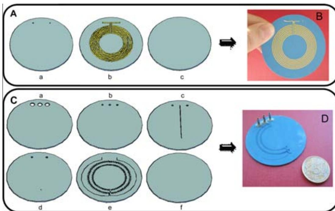
**Fig. 2.** Layer by layer design of both platforms integrating the LTCC microreactor. (A) Thermal platform; (a) top layer (4×); (b) screen-printed heater (1×); (c) bottom layer (4×). (B) Picture of the thermal platform fabricated. (C) Microfluidic platform; layers (a and f) were fabricated by duplicate; the microfluidic structure was embedded at layer (e). (D) Picture of the microfluidic platform, which includes an exposed section regarding the micromixer.
