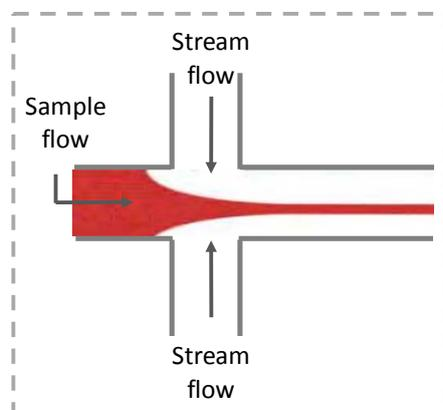
downstream (Figure 1.3).<sup>19</sup> In this way, the mixing path is reduced, since a very thin width central stream can be achieved. Moreover, the focused sheet can be deformed and moved out of the symmetry plane by changing flow rates of the side streams. This technique has been widely used in microfluidic applications to reduce mixing time.
