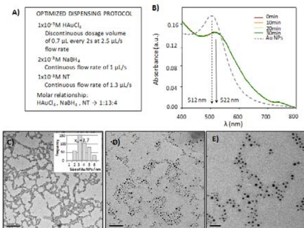
**Figure 4.20:** Results from the NT stabilized Au NPs, obtained in the **MR3** microreactor. **A)** Optimized chemical and hydrodynamic parameters. **B)** UV-Vis spectra recorded with time and its comparison with Au NPs. **C), D)** and **E)** TEM images and its correspondent histogram. **F)** DLS spectrum. **G)**  $\zeta$  potential measure.
