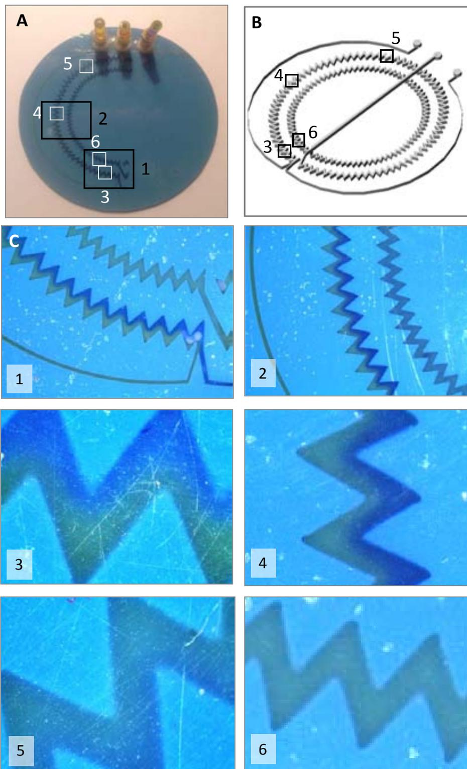
**Figure 5.21:** Fluidic/hydrodynamic qualitative visual characterization of the microfluidic system. **A)** Picture of the open to air microfluidic platform covered with a polymeric foil. **B)** Three-dimensional inner view of the microfluidic platform. **C)** Photographs corresponding to frames at different points of the micromixer.
