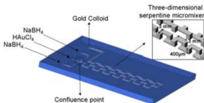
**Figure 2.** Microfluidic LTCC platform design for the synthesis of gold nanoparticles consisting of the concept of hydraulic focusing and a three-dimensional serpentine micromixer for the reagent mixture.
