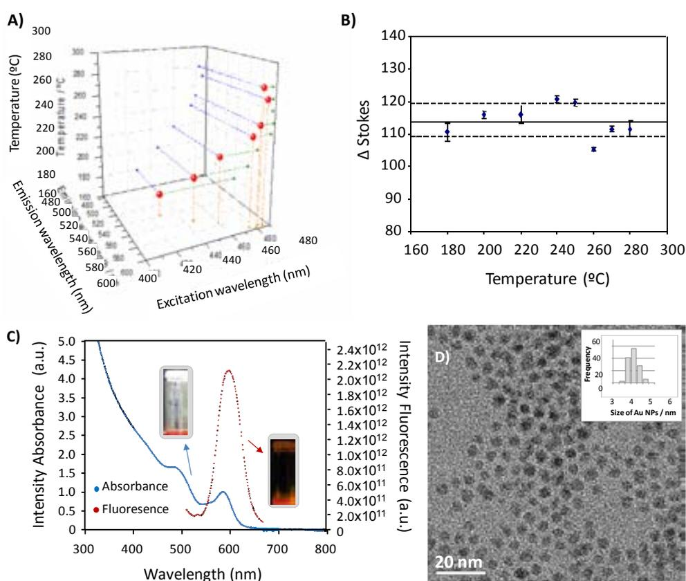
**Figure 5.25:** Results obtained for the synthesis of QDs in **MR6** with a 1:1 molar ratio of Cd:Se. **A)** Correlation between fluorescence emission peaks, excitation wavelengths and the different temperatures tested. **B)** Stokes shifts. Mean value of  $114 \pm 4.3$  nm. **C** and **D)** UV-Vis absorption band (blue, 485 nm), emission fluorescence (red, 596 nm) spectra and TEM image with its correspondent histogram of  $4.4 \pm 0.6$  nm QDs synthesized at 270°C.
