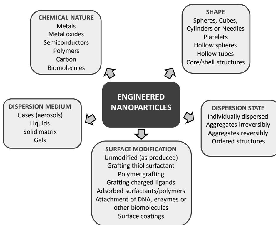
**Figure 1.10:** Diversity of engineered nanoparticles.<sup>82</sup>
