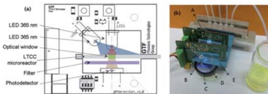
**Fig. 1** a) Scheme of the absorbance and fluorescent measurement set-up. b) Optical system and microreactor coupling. A: Absorbance LED, B: Fluorescence LED, C: high pass filter, D: PIN photodetector, E: ceramic microreactor.
