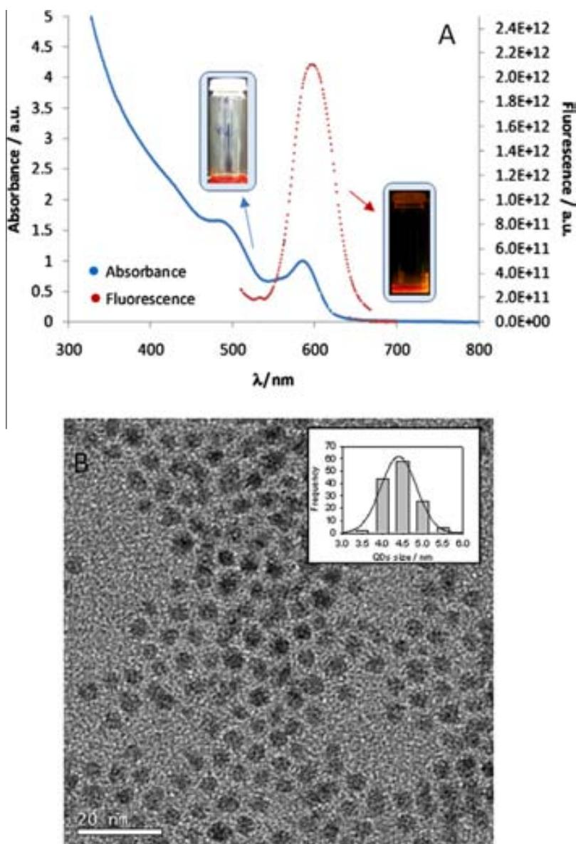
**Fig. 7.** (A) Absorbance (584 nm) and emission fluorescence (596 nm) spectra of the CdSe quantum dots synthesized in the modular microreactor. Images of the solutions of the obtained nanoparticles under visible and UV light can be also observed. (B) TEM image from the quantum dots synthesized.
