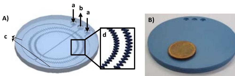
**Figure 5.17:** Schematic representation (A) and photograph (B) of the microfluidic platform; a: inlets, b: outlet, c: conditioner channels, d: amplification of a bi-dimensional micromixer.
