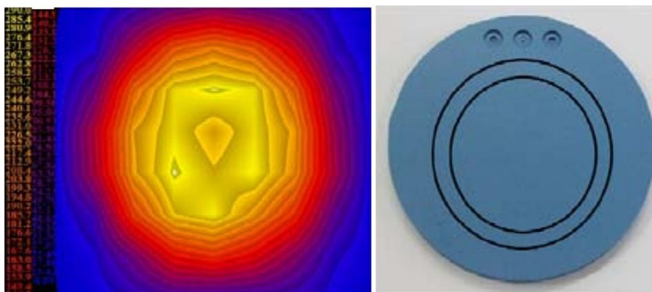
**Fig. S.1** (A) Isothermal map obtained for the microfluidic platform coupled to the thermal one; (B) image of the corresponding microfluidic module. The two black circles represents where the microfluidic channels are placed.
