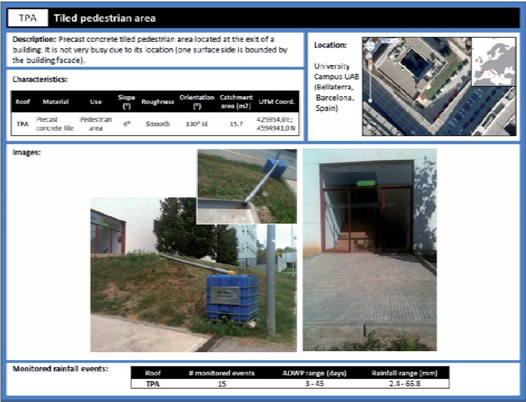
Figure 2.6. Main characteristics of the tiled pedestrian area study surface.
