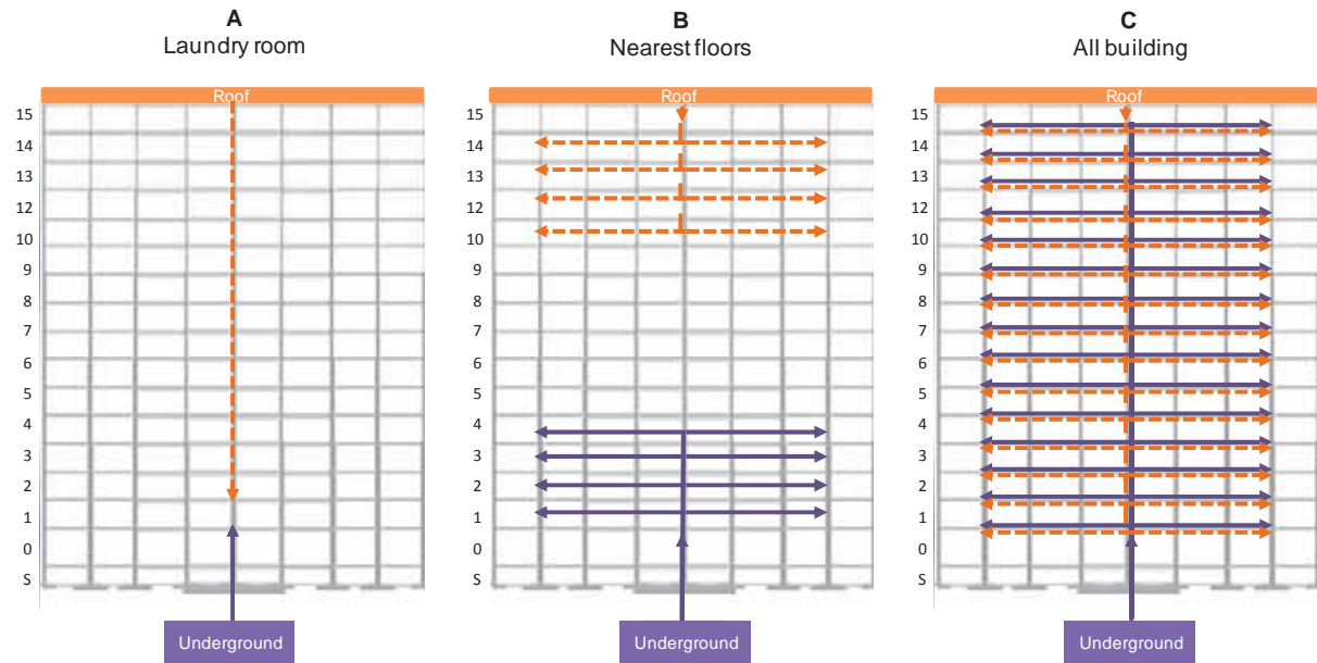
Figure 4.2. Front view of the three distribution strategies proposed for the roof (R) and underground (U) tank scenarios represented on the fifteen-story-building structure: A (laundry room), B (nearest floors) and C (all building)
