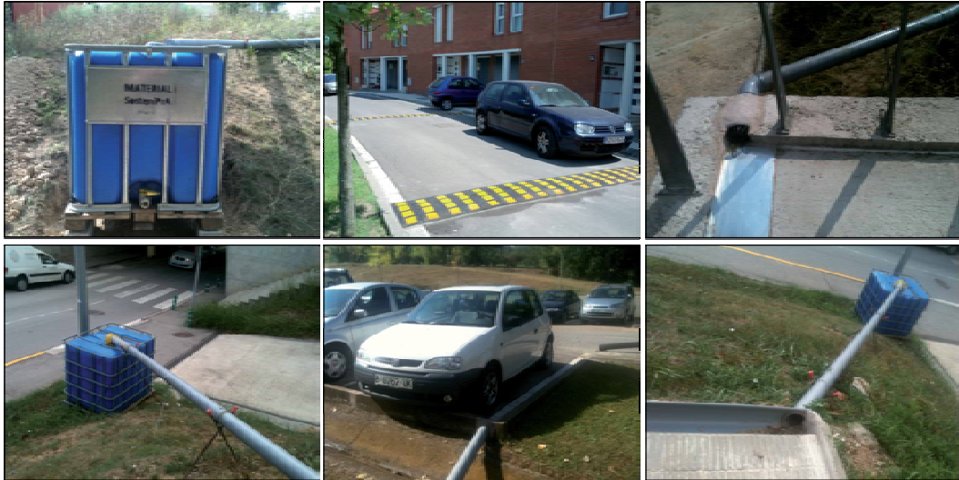
Figure 2.15. Rainwater harvesting system experimental installation at some sampling stations at the UAB campus.
