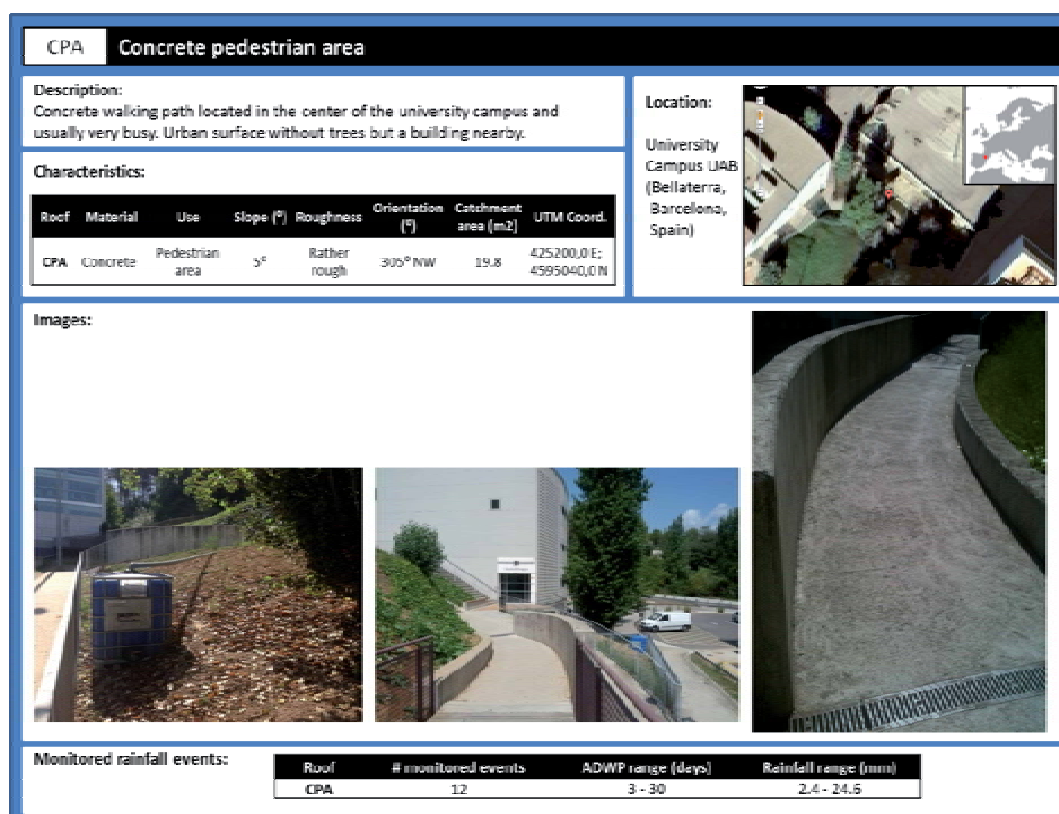
Figure 2.7. Main characteristics of the concrete pedestrian area study surface.
