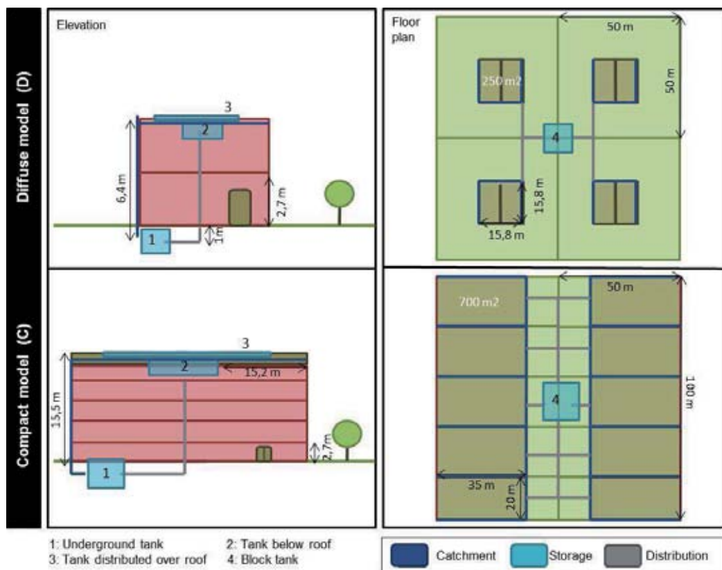
Figure 3.2. Characteristics of the study area based on the two urban densities defined and the location of the tanks at the building and block scale
