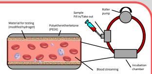
**Fig 3.** Blood will be recirculated through a circuit consisted of 3mm diameter silicone tubes, a section with valves that allow the affluence and exit of blood from a reservoir, a roller pump to regulate the blood flow and the incubator chamber. In order to maintain the pH value, CO2 and temperature constant, all the experiments will take place in an incubator<sup>4</sup>.
