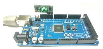
Fig. 7. Arduino Mega 2560 attached with a 433MHz receiver acting as the fixed receiver element.
