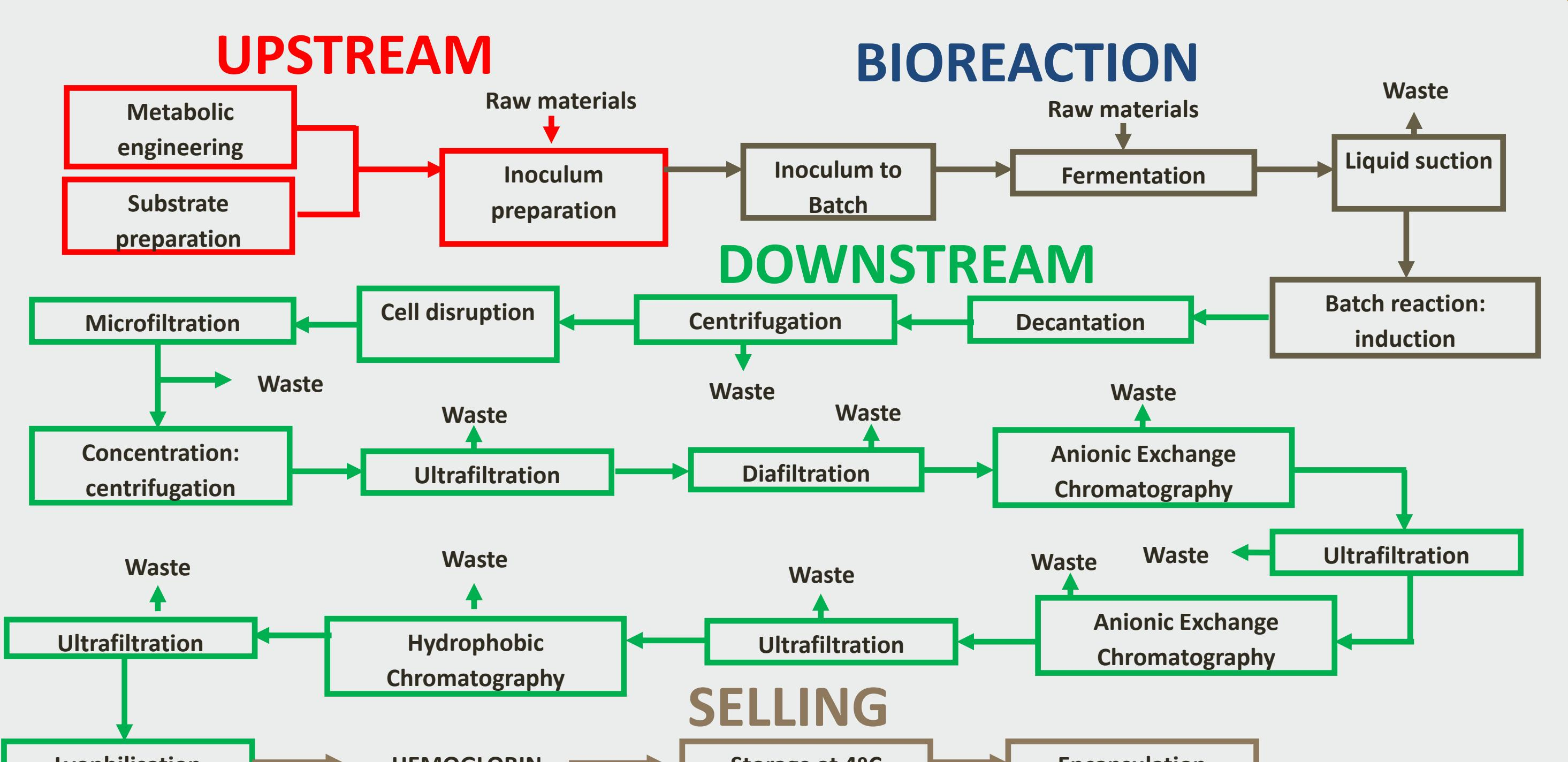
The complexity of the process is shown through the block diagram. The downstream process contains several stages to safeguard the purity of the protein and that is why it is the most expensive and difficult phase.
