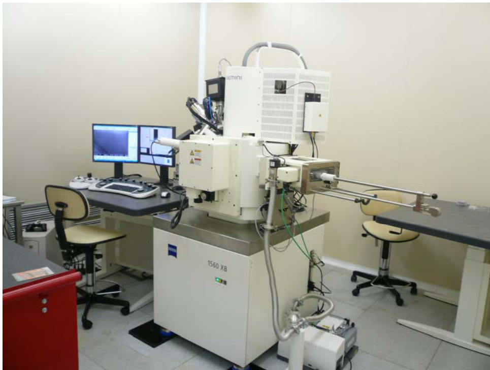
Figura 3.1.1_1. CrossBeam 1560XB al laboratori FIB de la ICTS (CNM-IMB)
