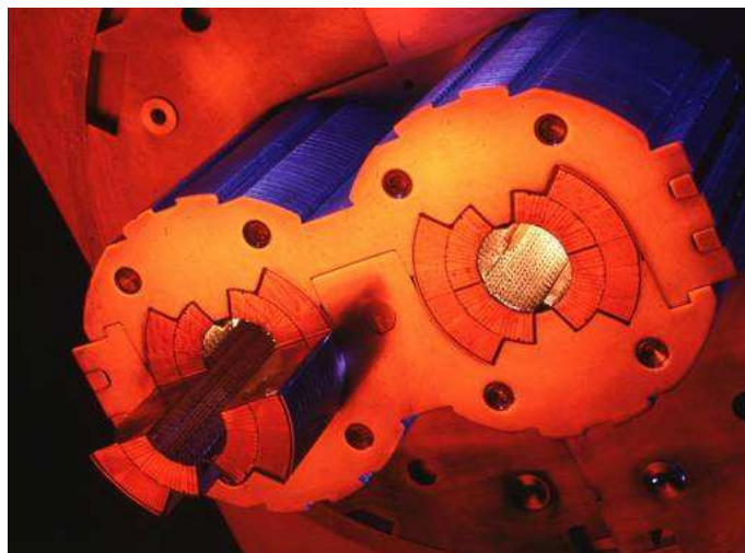
Figure 1.4: Close look of one of the main dipoles.
