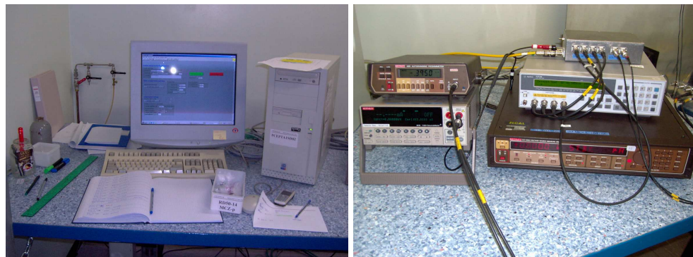
Figure 2.15: Computer used for monitoring the measurements and for data collection (left). Keithley485, Keithley 2410, Agilent 4263B, Keithley 237 and IV-CV coupling box (right).
