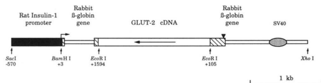
FIG. 1. Schematic representation of the RIP-I/anti-GLUT-2 chimeric gene used to create transgenic animals. The SacI/BamHI fragment (−570 bp to +3 bp) of the rat insulin promoter (21) was linked to a BamHI/XhoI fragment of the rabbit \beta -globin gene, which included the two last exons, the last intron, and the 3' region linked to the SV40 enhancer. The \beta -globin fragment and SV40 enhancer were included in order to ensure expression of the antisense transgene. An EcoRI fragment (+105 bp to +1594 bp) of the GLUT-2 cDNA (19) was introduced in reverse orientation at the EcoRI site of the second exon of the \beta -globin gene. The 4.26-kilobase pair SacI-XhoI fragment containing the entire chimeric gene was used to obtain transgenic mice. The triangle (▼) represents the polyadenylation signal from the \beta -globin gene.
