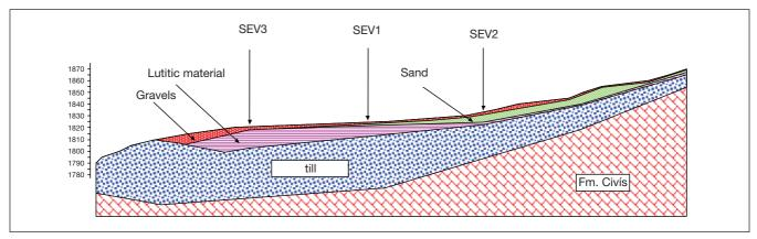
Figure 2. Vertical Electric Soundings (SEV) .
