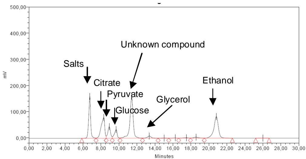
Chromatogram with the unknown peak at retention time of 11.5 min in a HPLC
