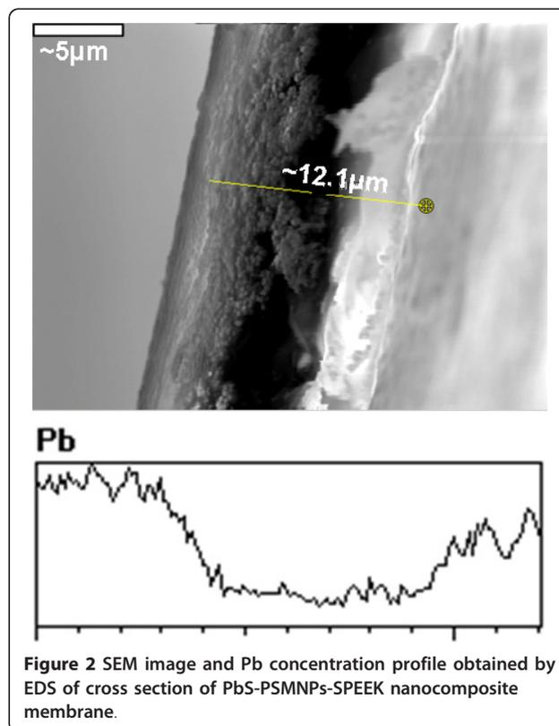
Figure 2 SEM image and Pb concentration profile obtained by EDS of cross section of PbS-PSMNPs-SPEEK nanocomposite membrane.
