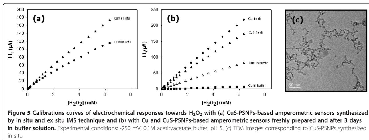
has been successfully proved. The resulting amperometric sensors showed a relatively high sensitivity and a much higher stability against oxidation than those prepared using Cu-PMNCs.
