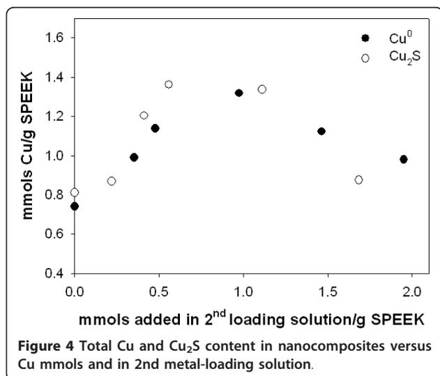
**Figure 4** Total Cu and  $\text{Cu}_2\text{S}$  content in nanocomposites versus Cu mmols and in 2nd metal-loading solution.
