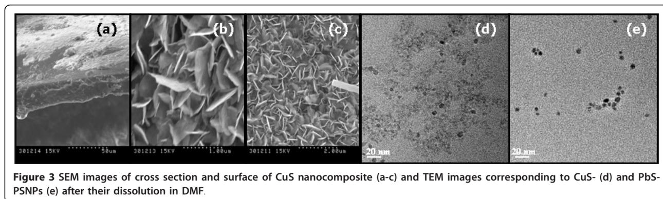
**Figure 3** SEM images of cross section and surface of CuS nanocomposite (a-c) and TEM images corresponding to CuS- (d) and PbS-PSNPs (e) after their dissolution in DMF.
