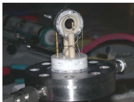
Figure 4. Internal view (upside down) of a prototype of half electrochemical cell
