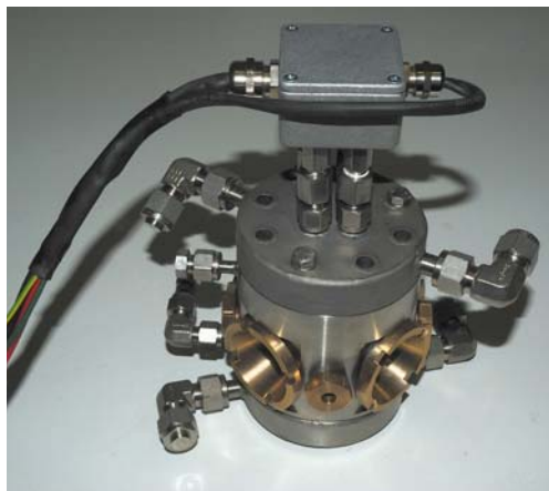
Figure 1. External view of the multi-purpose in-situ cell for solid-gas catalysis.
