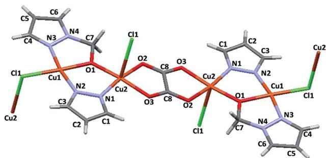
**Fig. 1** X-Ray structure of the  $[\text{Cu}_4\text{Cl}_2(\text{Ox})(\text{L1})_2(\text{L2})_2]$  complex, where  $[\text{Cu}_2\text{Cl}(\text{Ox})_{0.5}(\text{L1})(\text{L2})]$  is the basic monomeric unit of this polymeric chain. Colour scheme: copper, orange; oxygen, red; chlorine, green; nitrogen, blue and carbon, grey.
