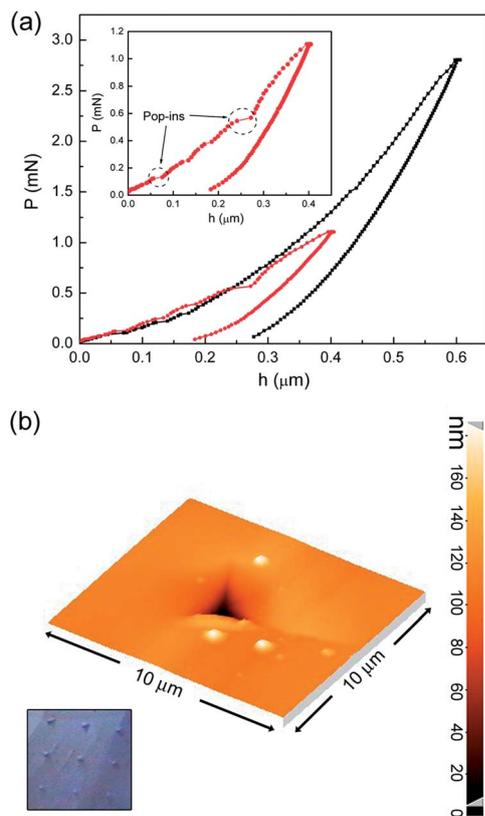
Fig. 3 (a) Representative nanoindentation curves performed perpendicular to the crystal sheet, and up to maximum loads of 1.2 mN (red line) and 2.8 mN (black line). (b) Atomic force microscopy and optical (inset) images of an indentation performed using a maximum load of 2.8 mN.
