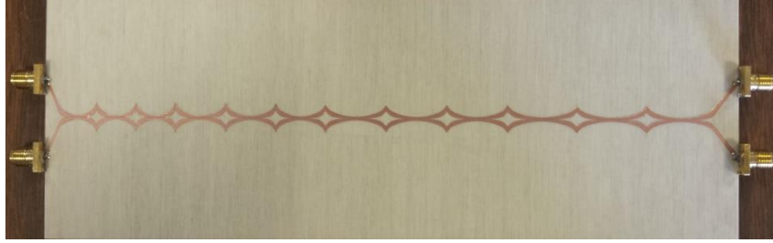
Fig. 6. Photograph of the 5 GHz multi-tuned EBG-based differential microstrip line centered at f_0 = 5 GHz.
