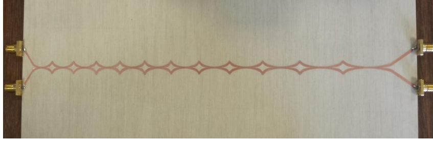
Fig. 3. Photograph of the 5 GHz chirped-EBG based differential microstrip line with wideband common-mode rejection.
