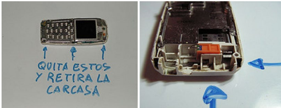
Figure 4. By Obsoletos with CC BY-SA 3.0 ES licensing. The written instruction says, ‘unscrew these and remove the cover’.
