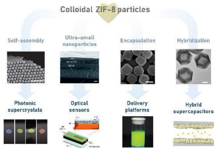
Fig. 9. Diagram of the perspective applications of colloidal ZIF-8 in the different forms discussed in this review. Scale bar (all micrographs): 1 \mu\text{m} . 15,18,39,49
