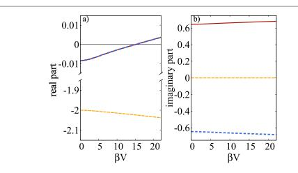
**Figure E1.** Eigenvalues of  $J_0$  evaluated at the steady state as a function of the applied bias voltage. As *V* is increased the two complex conjugated eigenvalues (solid red and dotted blue) become purely imaginary at a critical value of  $\beta V_{cr} = 15$ , which denotes the bifurcation point and the stability of the fixed point changes. Further increase of *V* results in a stable limit cycle and an unstable fixed point.
