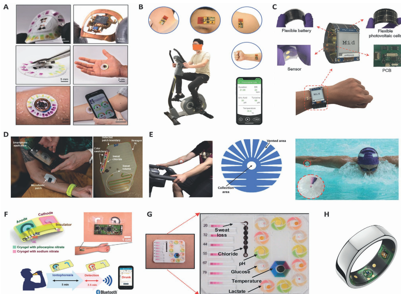
Figure 1. Integrated diagnostic devices for sweat analysis. A) Battery-free hybrid microfluidic device for electrochemical, colorimetric, and volumetric sweat analysis. Reproduced with permission. [26] Copyright 2019, American Association for the Advancement of Science. B) Laser engraved wearable device for uric acid and tyrosine detection for gout and metabolic disorders monitoring. Reproduced with permission. [36] Copyright 2020, Nature. C) Self-powered smartwatch for semi-quantitative continuous glucose monitoring. Reproduced with permission. [40] Copyright 2019, American Chemical Society. D) Skin-interfaced microfluidic system that can capture sweat rate and electrolyte concentration to provide personal sweat profile. Reproduced with permission. [44] Copyright 2020, American Association for the Advancement of Science. E) Waterproof sweat patch for sweat collection, biomarker analysis, and thermography in aquatic settings. Reproduced with permission. [32] Copyright 2019, American Association for the Advancement of Science. F) Iontophoretic tattoo-based sensing for alcohol monitoring. Reproduced with permission. [45] Copyright 2019, American Chemical Society. G) Multifunctional microfluidic system for colorimetric measurement of sweat parameters and temperature. Reproduced with permission. [30] Copyright 2019, American Chemical Society. H) Smart ring can track the key signals from the body like heart rate, heart rate variability, temperature which has been recently offered by NBA to the players for “early illness detection monitoring” during coronavirus pandemic. Reproduced with permission. [21] Copyright 2020, OuraRing.
