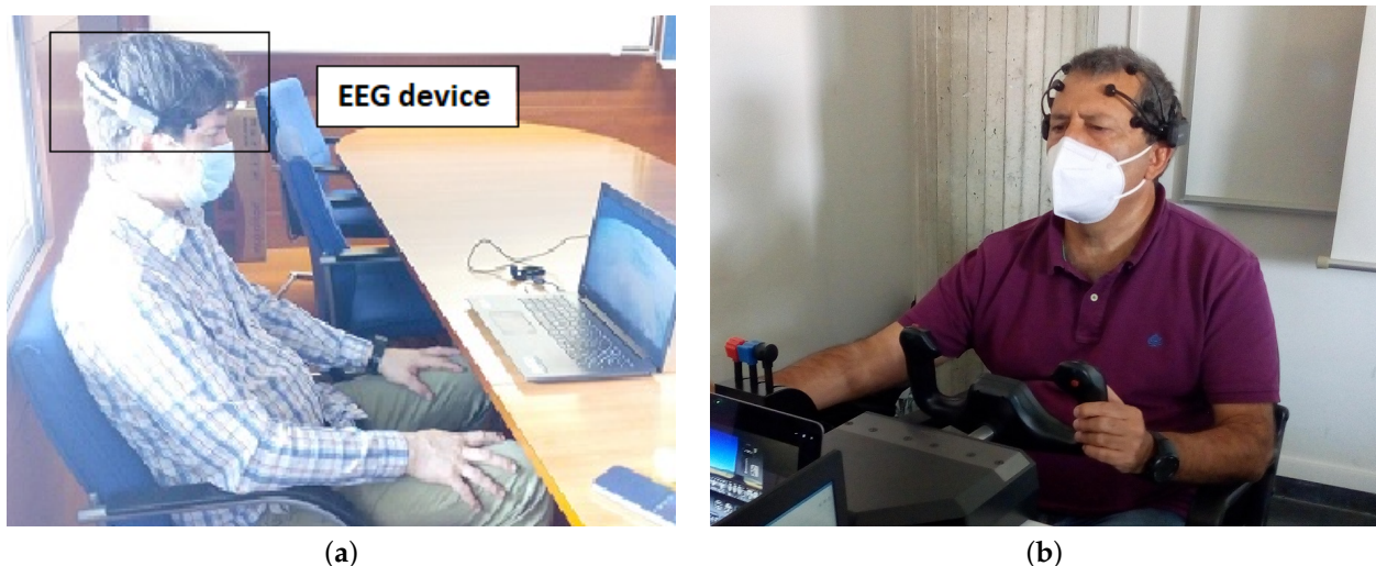
Figure 1. Data collection with Emotiv Epoc+ headset. (a) A volunteer during a n-back-test and (b) a pilot during simulated flight session.
