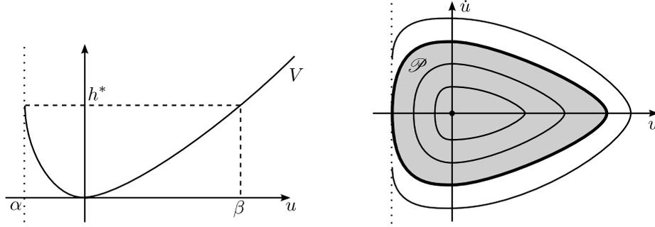
FIGURE 1. On the left, potential function with a weak singularity at  $x = \alpha$ . On the right, the phase portrait of the potential system. The grey region corresponds to the period annulus. Its outer boundary is emphasized in bold.
