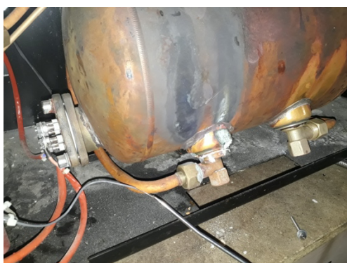
Fig. 2. Copper boiler and the effect of corrosion due to hard water
