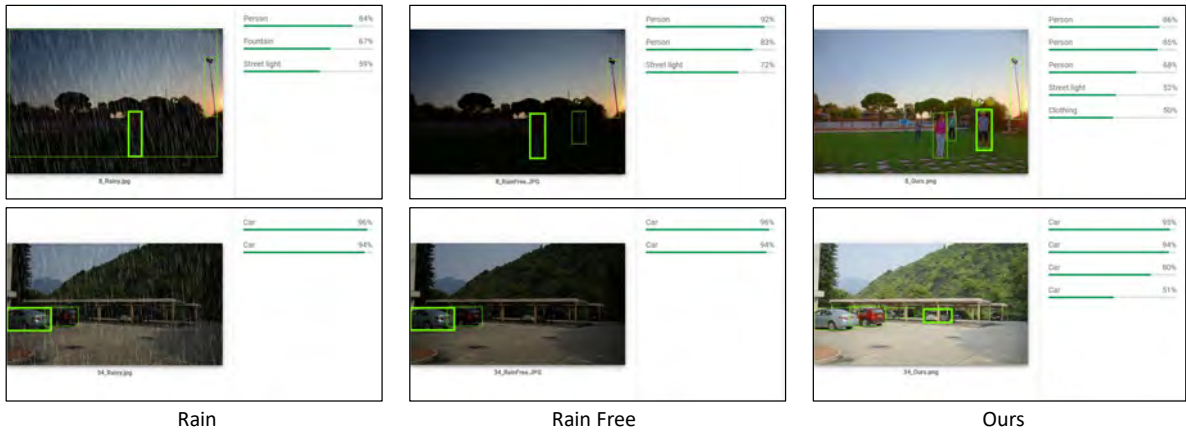
Figure 12: The restoration results are tested on the Google Vision API. Left: object recognition result in the rain image. Middle: object recognition result in the rain free image. Right: object recognition result in the image restored using our method.
