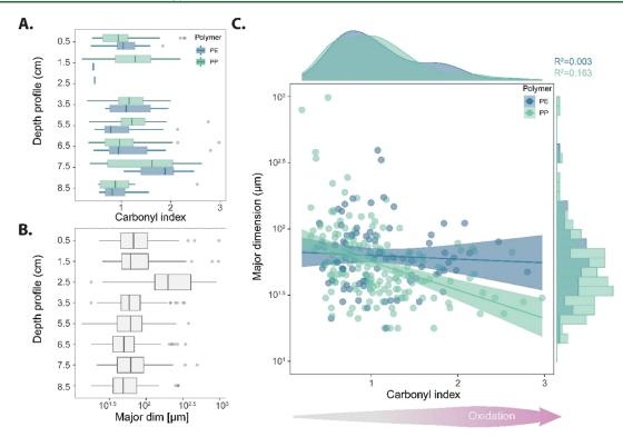
**Figure 4.** Summary of the MP weathering status and size variability in the sedimentary record A. Boxplot of the carbonyl index in the sediment profile classified as polyethylene (dark blue) and polypropylene (light blue). (B) Boxplot of the size variability (y-axis logarithmic scale) in the sediment core. C. Increase of the oxidation status of the polymers, measured as carbonyl index, as the particle size decreases (y-axis logarithmic scale).
