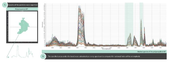
**Figure 3.** Illustrative example of the calculation of the carbonyl index for a polypropylene particle. From left to right, the image on the visualization of a particle, every pixel represents a collected spectrum. Spectra were exported from the siMPle software and treated in SpectraGryph 1.2.15 where the area below the band was computed.
