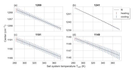
**Figure 3.** Temperature dependence of different bands located at: (**a**) 1269, (**b**) 1241, (**c**) 1191, and (**d**) 1149 cm<sup>-1</sup>. The sample has been heated (red) and cooled (blue) over the temperature region between 283 and 373 K. Data points are shown with numerical error from the fit. A linear model has been fitted (grey lines) with the resulting slopes listed in Table 1.
