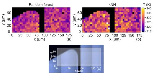
**Figure 6.** Hyperspectral images showing the temperatures predicted by the (**a**) random forest and (**b**) k-NN machine learning algorithms. The regions of the metallic gold wire are masked in black. (**c**) Optical image with the metallic gold coating (black) on a PMMA thin film (blue) and the sampled area of the hyperspectral imaging in white.
