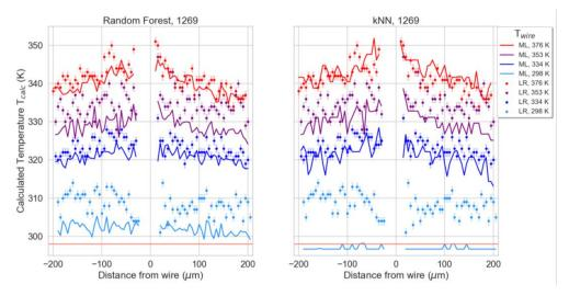
**Figure 5.** Temperatures ( $T_{calc}$ ) predicted with linear regression (LR) for the peak at 1269 cm<sup>-1</sup> indicated by "•"-markers and temperatures predicted by the machine learning (ML) approaches indicated by lines, using the random forest (**left**) and k-NN (**right**) algorithms. The data were measured with the gold wire temperature (Twire) at room temperature (298 K) and heated to 334, 353, and 376 K. Room temperature is indicated with horizontal red lines.
