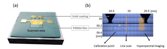
**Figure 1.** (a) Schematic representation of the heating device deposited on top of the polymer film. (b) Optical transmission image of the sample, showing the metallic wire in black with the three infrared measurement areas highlighted in orange.
