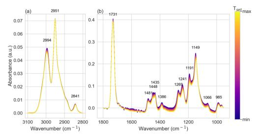
**Figure 2.** Infrared absorption spectra of PMMA measured with variable temperature from 283 and 373 K in 3 K steps. (**a**) All spectra have been baseline corrected in the region of the C-H vibrational peaks between 3100 and 2800 cm<sup>-1</sup> and (**b**) the fingerprint region between 1800 and 950 cm<sup>-1</sup>.
