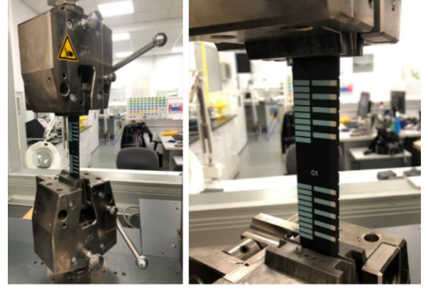
Fig. 10. Photographs of the encoder, with one layer of conductive silver ink coated with a layer of green dielectric ink, being stressed mechanically.
