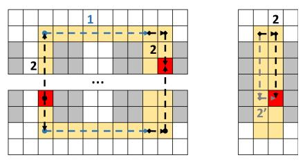
**Figure 5.** The movement around the racks (1) is the shortest, trivially. The movement within the aisle (2) is also minimal. Other paths within the aisle can be found (2') but the length would be the same or larger.
