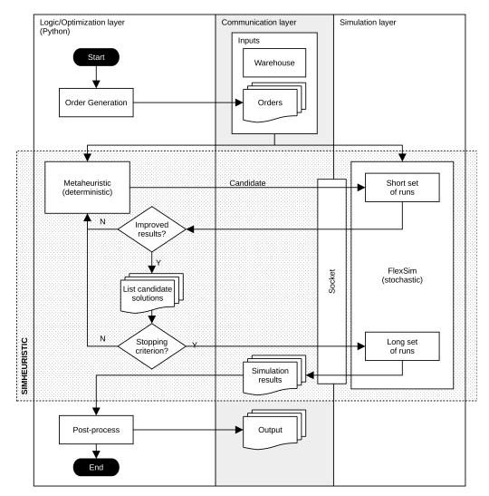
Figure 4. Description of the simheuristic framework logic.
