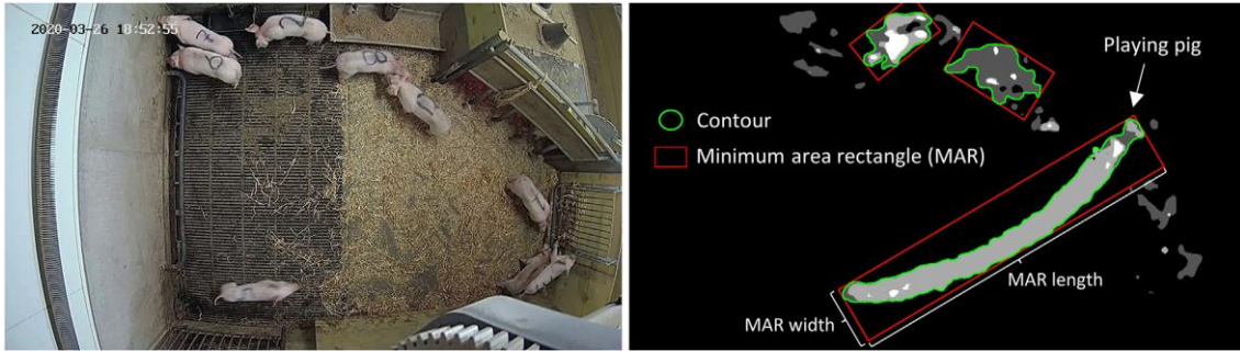
Fig. 1 e Example of a movement map including a pig performing locomotor play. Left: first raw frame (out of 15) used to construct the movement map. Right: 15 frames (1 s) movement map with the green solid lines representing the contours detected and the red rectangles representing the minimum area rectangle for each contour.
