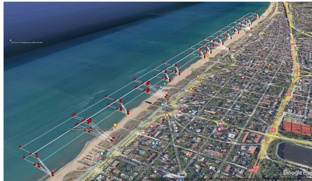
Figure 2. Corridor-based airspace structure used in the Spanish demonstrations in the CORUS-XUAM project.
