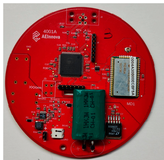
Figure 11. The main board is soldered with all components ready for testing.
