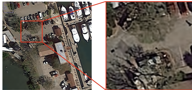
Fig. 12. Visual example of decompressed image and specific zoom area presented in Zhang et al.'s [25] work. This image was compressed at 0.096 bps (0.28 bpp) obtaining a reconstruction quality of 29.65 dB PSNR.
