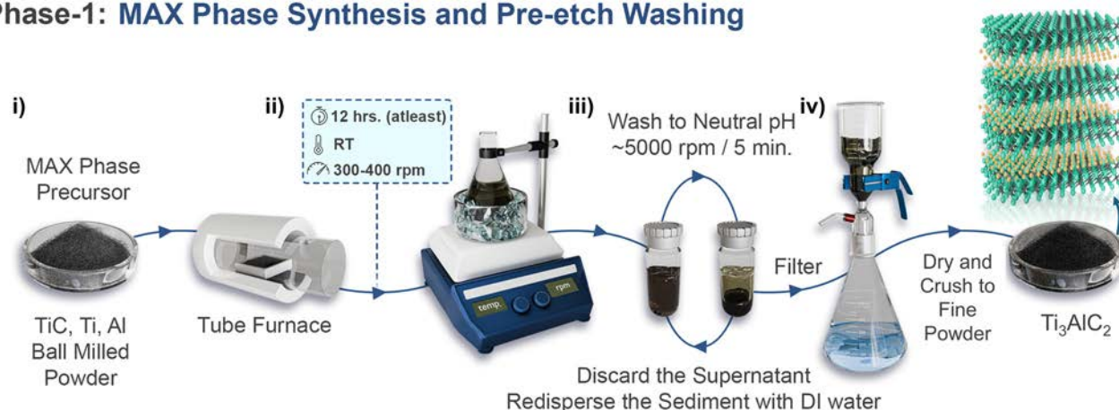
Scheme 2 (i) Schematic of the laboratory setup used for synthesis of MAX phase. (ii) Experimental setup and parameters required for pre-etch HCl washing. (iii) Depiction of repeated centrifugation for pH control. (iv) Depiction of the vacuum filtration assembly to collect the MAX powder.
