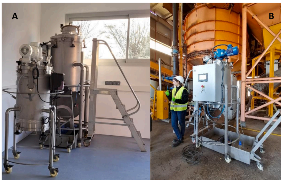
Fig. 1. Images of the bioreactors. A) R100 (in front) and R290 (back) at GICOM's facilities in UAB; B) R290 in Granollers (Barcelona, Spain) biowaste treatment plant during the execution of the experiments reported herein.
