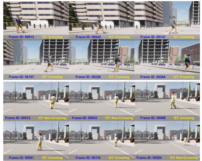
Fig. 2. Summary of two videos from PedSynth. Top rows: a pedestrian crosses the road perpendicularly to the ego-vehicle moving direction. Bottom rows: a pedestrian changes the intention of crossing the road at mid-lane. In both examples, the pedestrians enter the road at locations that are not enabled for crossing. GT stands for ground truth ( i.e. , C/NC label).
