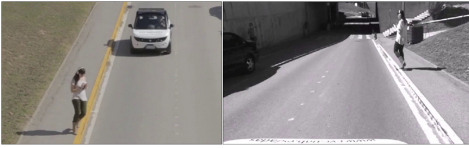
Fig. 1. Left: a distracted pedestrian intends to cross the road through a non-zebra crossing while listening to music, as a vehicle approaches. Right: an image captured by the vehicle's onboard camera. Autonomous vehicles must detect the pedestrian's intention to cross before it occurs to execute a safe and comfortable braking, similar to how a human driver would react.
