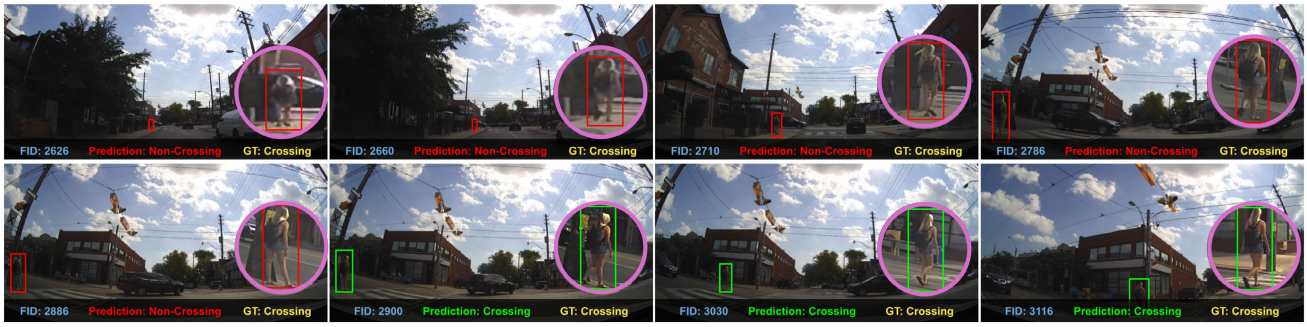
Fig. 5. Discrepancies between human-provided C/N labels and pseudo-labels in the PIE training set. The naming and color conventions follow those in Figure 4. Please refer to the main text for further discussion on this figure.
