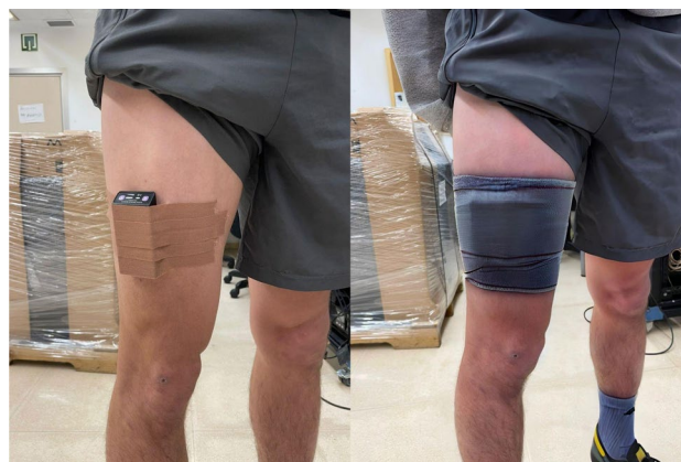
Fig. 1 The PortaMon device was placed and secured on the vastus lateralis of the right leg
