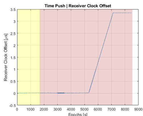
Figure 2. The receiver clock offset was provided by the NovAtel G-III receiver during the time-push attack.
