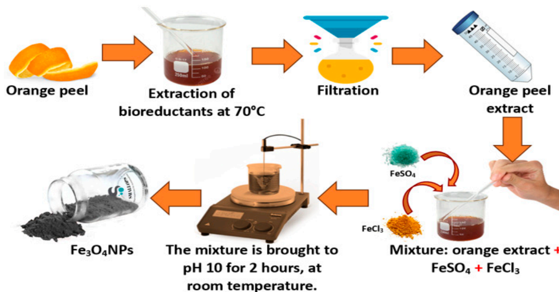
Scheme 1. Fabrication procedure of Fe 3 O 4 NPs using orange peel extracts by eco-friendly green synthesis method.
