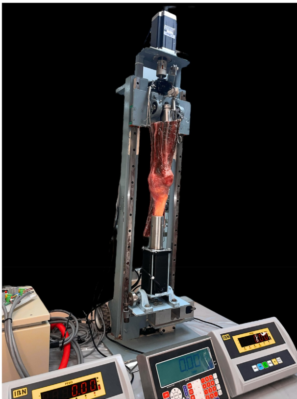
Fig. 1. Photograph of the setup of the human cadaveric knee assembled in the biomechanical device used in the present study.
