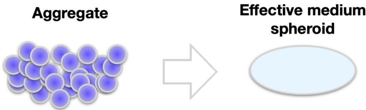
Fig. 2 A cartoon showing the concept of the spheroidal analog approximation of a porous aggregate
