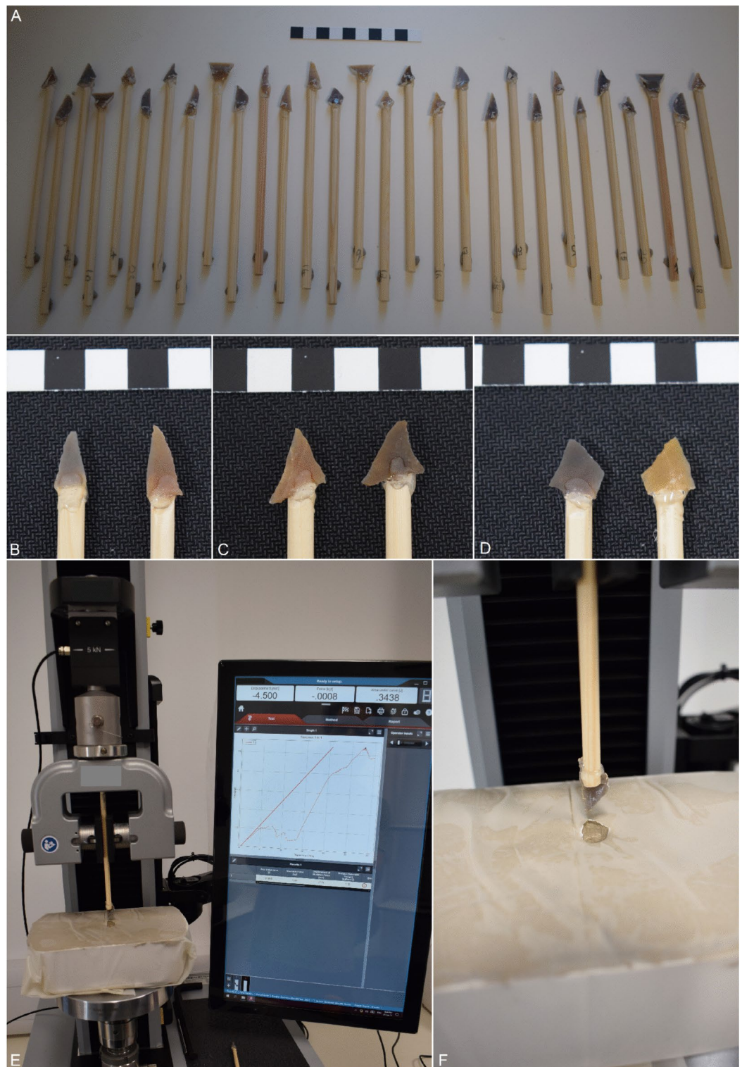
Fig. 3. The sample of replica geometric microliths hafted to the wooden dowels (a), three pairs of geometrics prior to testing (b–d), the Instron device and wider experimental set-up, including an exemplar force–deformation curve (e), and a close-up of the experiment post-test (f).
